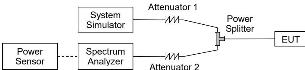
The EUT is coupled to the Spectrum Analyzer (SA) and the System Simulator (SS) with Attenuators through the Power Splitter; the RF load attached to the EUT antenna terminal is 50Ohm; the path loss as the factor is calibrated to correct the reading. The EUT is commanded by the SS to operate at the maximum output power i.e. Power Control Level (PCL) = 5 and Power Class = 4. A call is established between the EUT and the SS.
