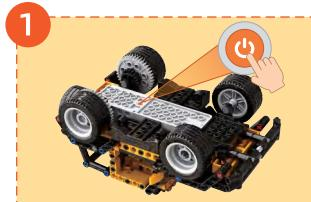
Short press the power button of the control module. The LED lights will flash blue every 1 second.
