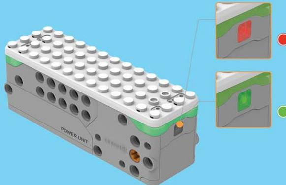
APP control mode pairing: shortly press the power button and turn on the power of the main control unit, it will flash green after 10 seconds, Turn on your device' s Bluetooth and go to the Bluetooth pairing page Bringing your device closer to the main control unit, and the pairing completed automatically.
