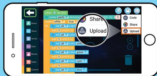
After you own program is completed, click the Upload button in the APP. Turn off the power of the main control unit, then press and hold for 5 seconds to turn it on. The robot starts off-line mode and runs automatically according to the uploaded program.
