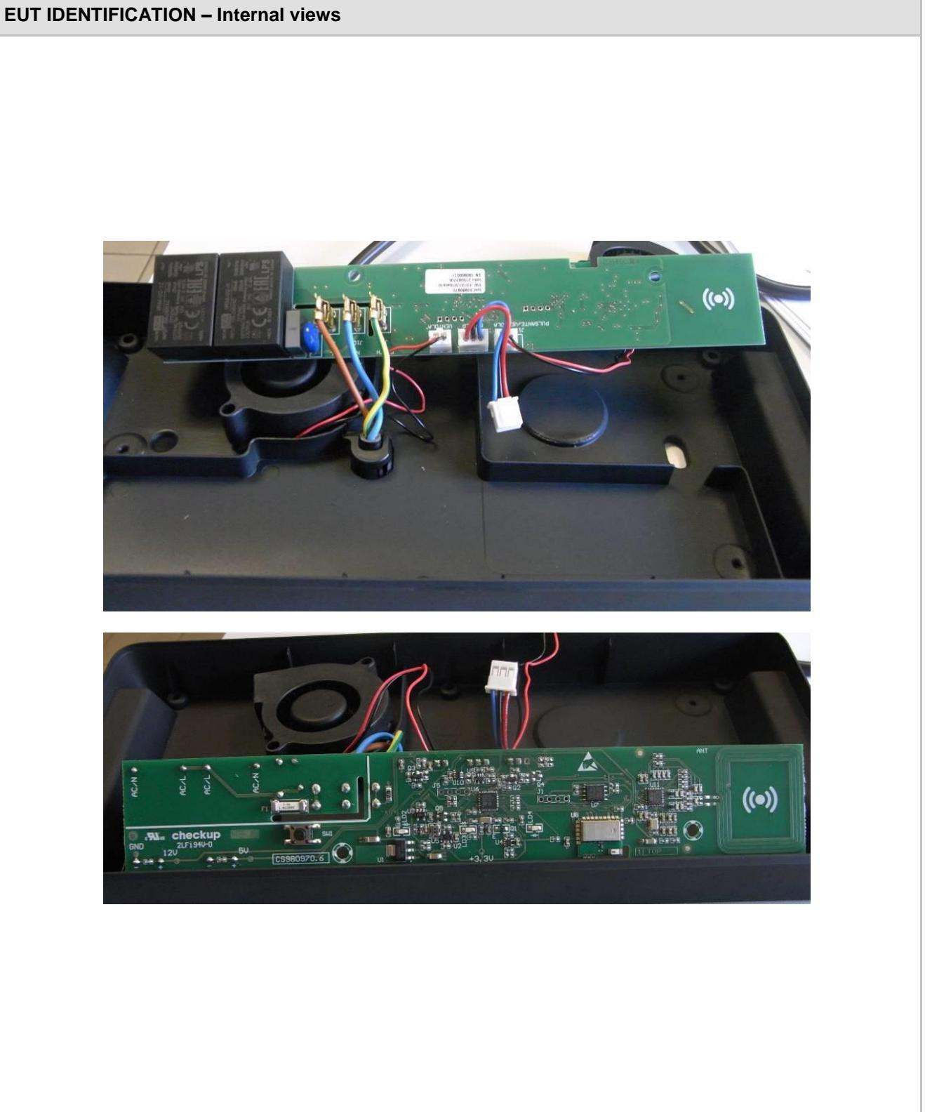
**EUT IDENTIFICATION – Internal views radio module**
