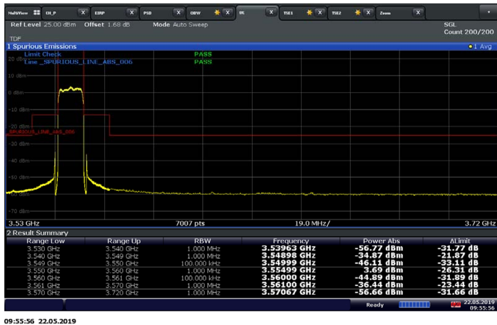
LTE Band 48 / 10 MHz / 16QAM
