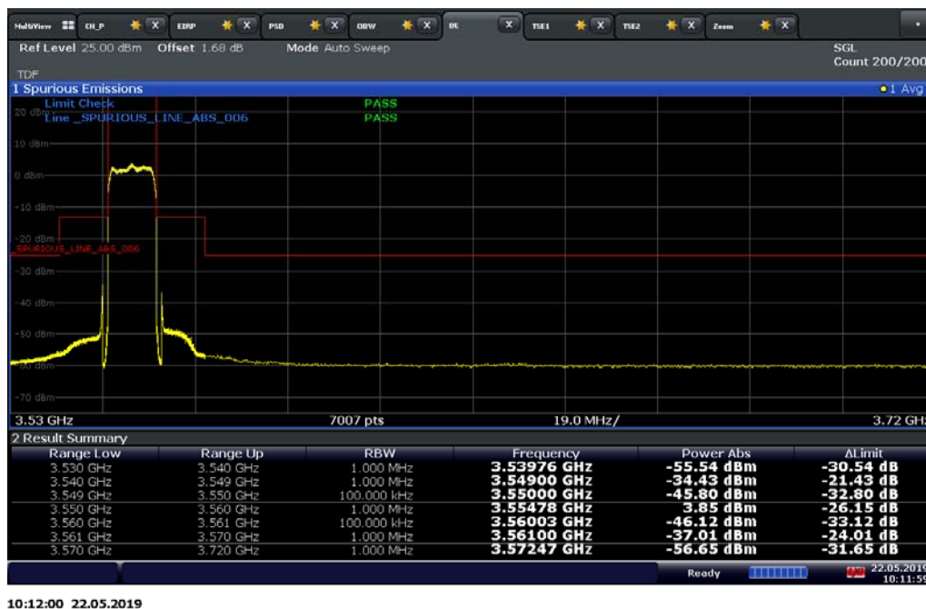
LTE Band 48 / 10 MHz / 16QAM
