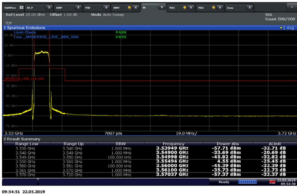
LTE Band 48 / 10 MHz / 16QAM
