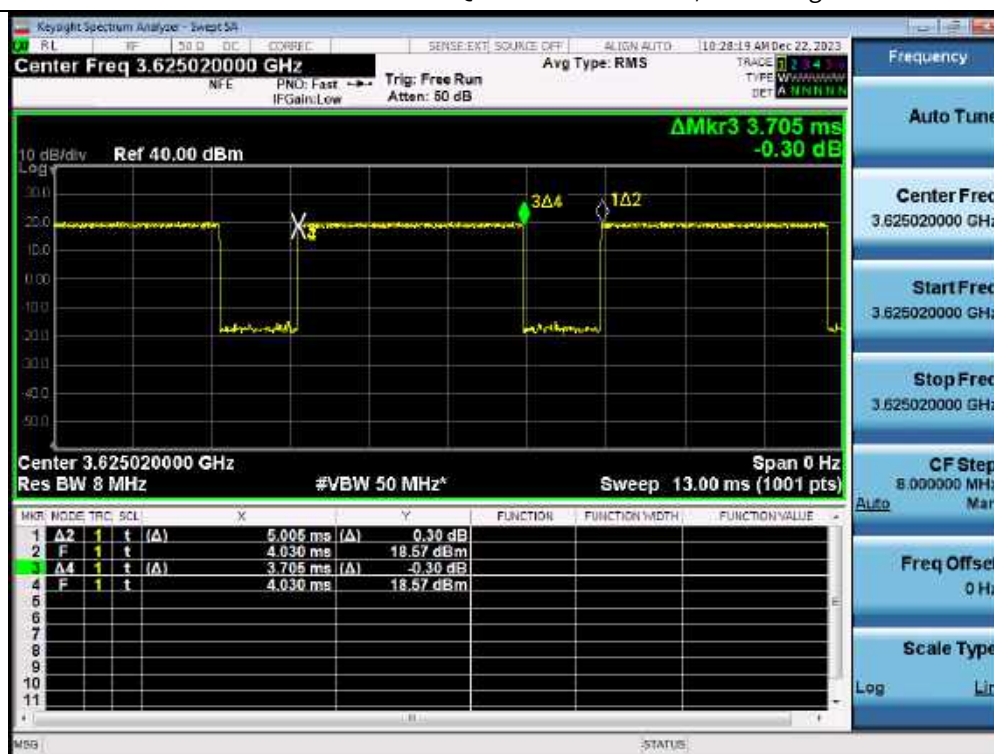
Measurement Result of QC-336A Transmit On/Off Timing
