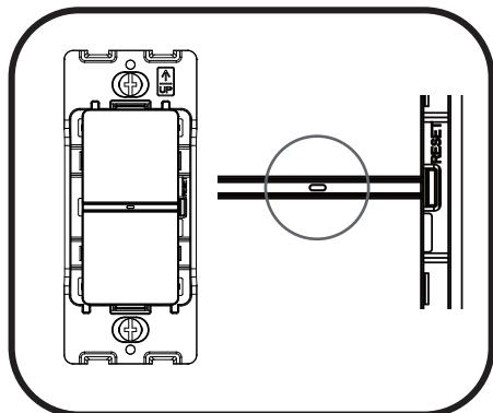
**1** The device's LED flashing on for 2 seconds every 30 seconds indicates that the batteries need to be replaced.
