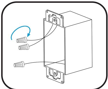
4 Reconnect wires (previously connected to wall switch) with wire nuts.
