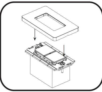
4 Install the main body of the device into the back housing.
