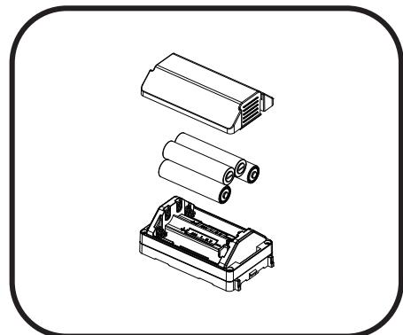
**3** Separate the battery cover from the device. Replace the batteries with AAA batteries. All batteries need to be replaced at the same time.
