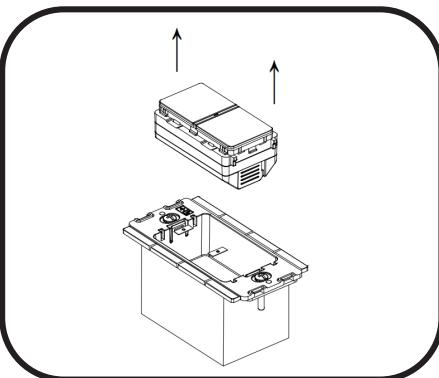
**2** Remove the device from the back housing.
