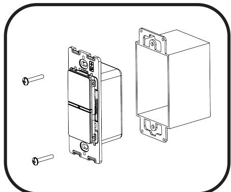
6 Install the back housing(s) of the wall dimmer(s) into the wall box.
