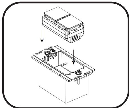
**4** Install the main body of the device into the back housing.
