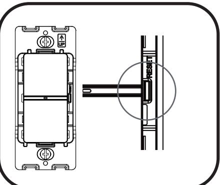
To reset the network of the device, remove the faceplate from the device. Then press and hold the reset button for 5 seconds. Install the faceplate back onto the device. Press either dimming up or down button to enter the pairing mode to join the device to a network.
