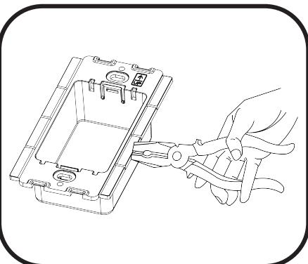
5 For proper installation into a dual gang junction box, the tabs between adjacent back housings must be removed. Carefully observe the correct orientation (the UP arrow should be in the upper right corner on each back housing). After double checking the product orientation, break off the necessary tabs using pliers.
