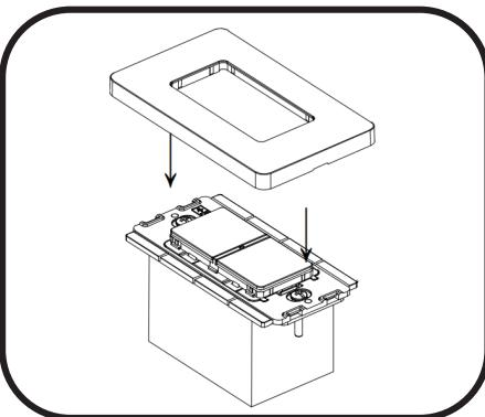
**5** Install the faceplate onto the device. The device will rejoin its network automatically.
