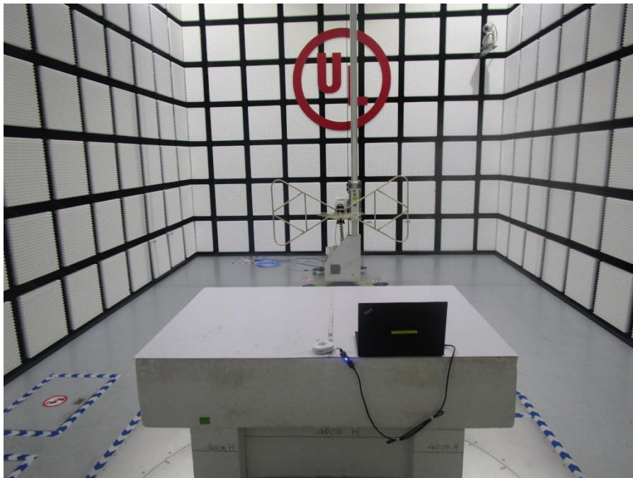
RADIATED RF MEASUREMENT SETUP (30MHz~1GHz)
