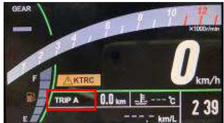
Short press of left button to change the ODO display to TRIP A display , then long press of left and right buttons to enter Menu.
