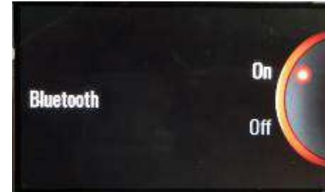
Short press of left button to move the selection to ON then short press of right button to confirm.
