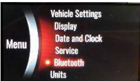
Short press of DOWN SW to move the selection to Bluetooth then short press of Select SW to enter Bluetooth setting.
