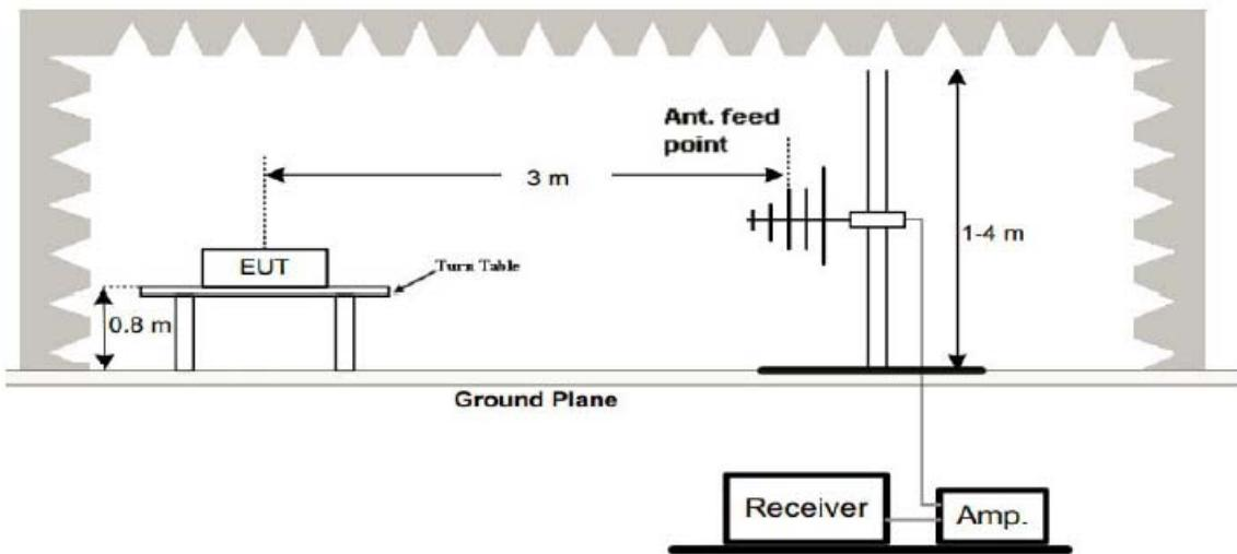
(3) Radiated Emission Test-Up Frequency Above 1GHz
