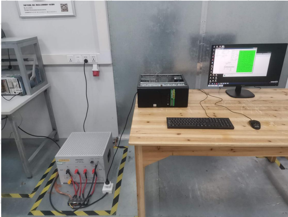
Photo of Power Line Conducted Emission Test
