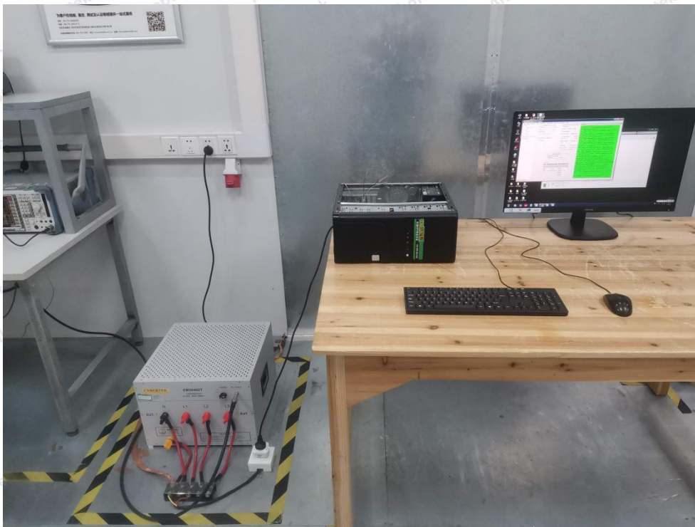
Photo of Conducted Emission Test
