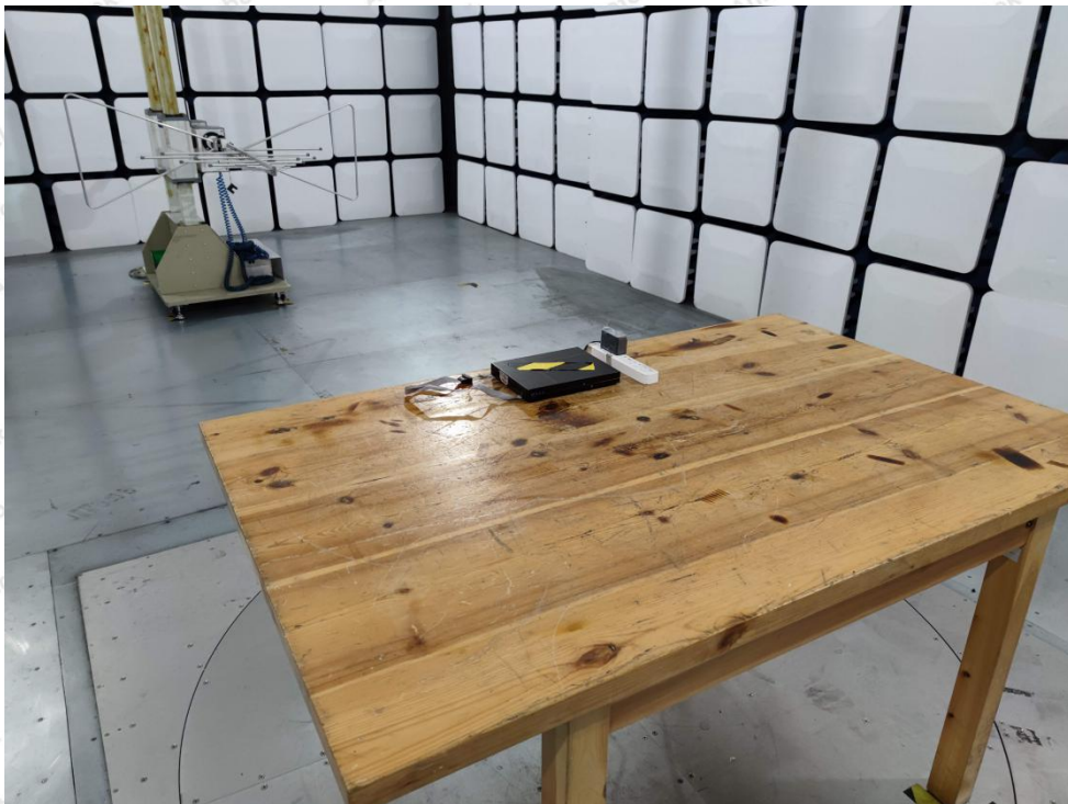
Photo of Radiation Emission Test
