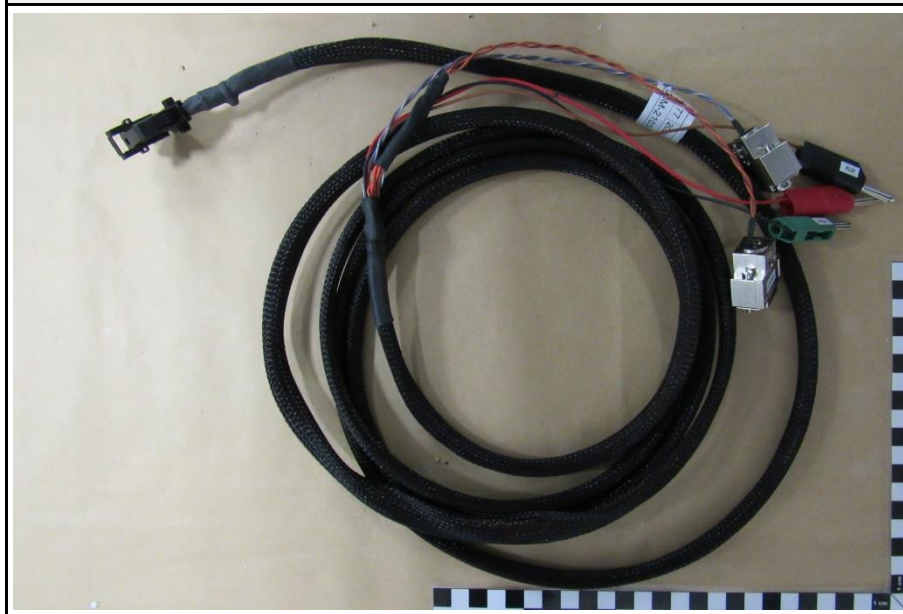
AE: Power and CAN cable
