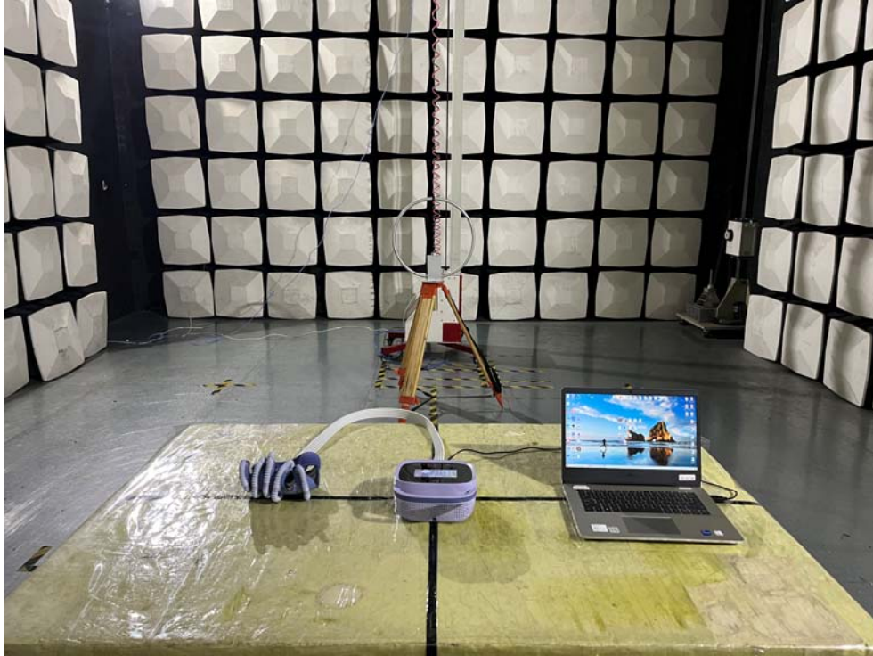
Test Photo Radiated emission (Below 30MHz)
