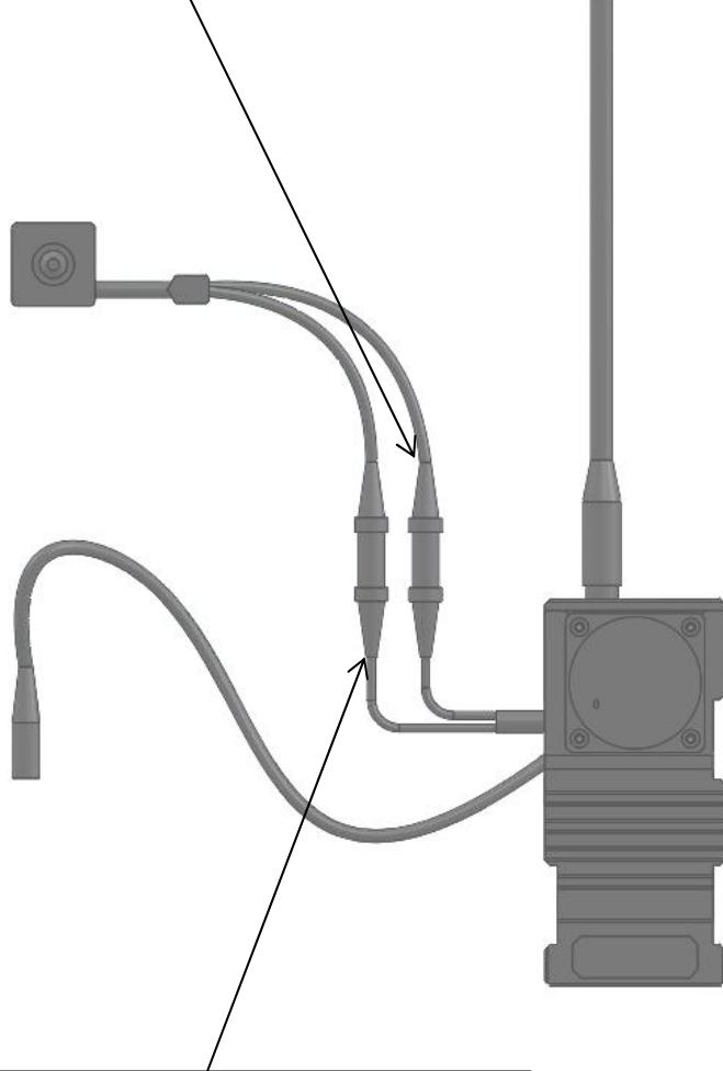
ALIGN THE RED DOTS WHEN PLUGGING.
