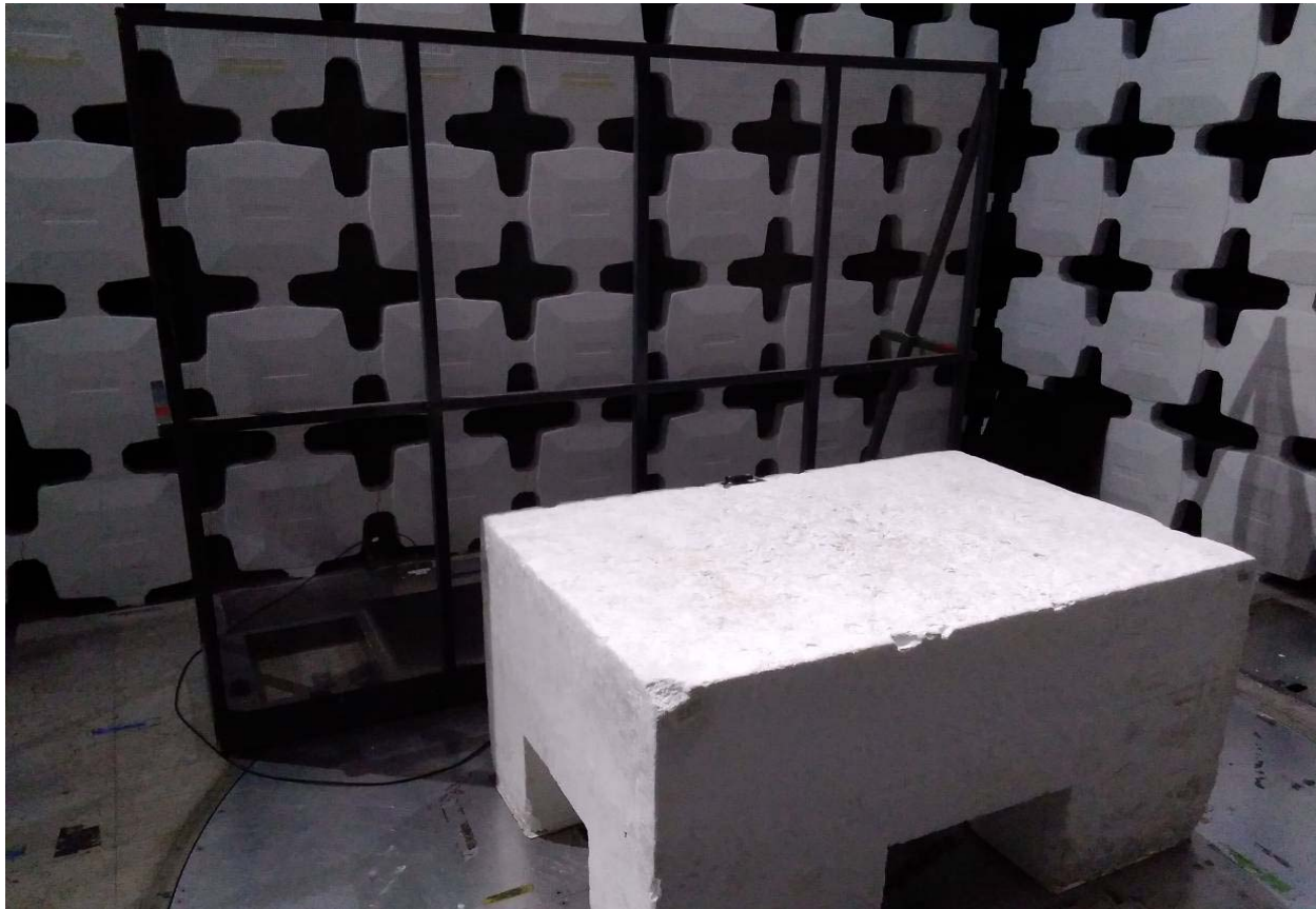
Test Configuration Photograph #1 (Conducted Emissions - Power Port)
