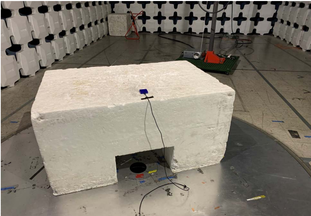
Test Configuration Photograph #2 (Radiated Emissions - Below 30 MHz)
