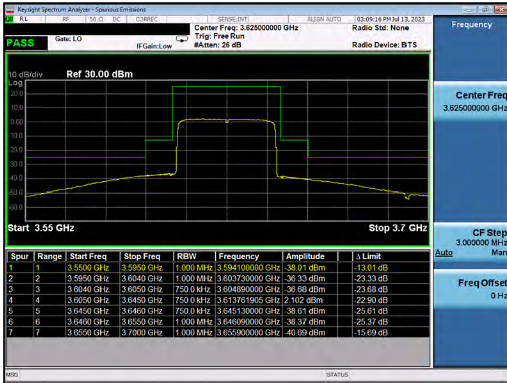
Plot 7.207. Conducted Band Edge Plot (40MHz, QPSK, Mid Channel, Ch.B)
