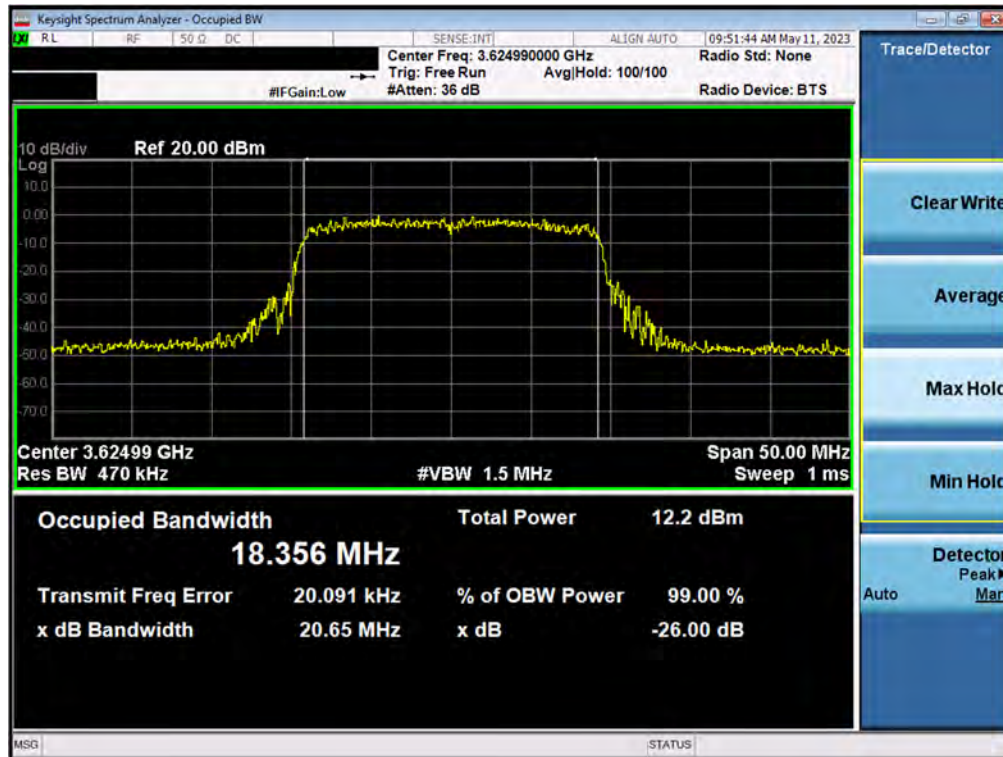
Plot 7.43. Occupied Bandwidth Plot (20MHz 64-QAM – Ch.A)
