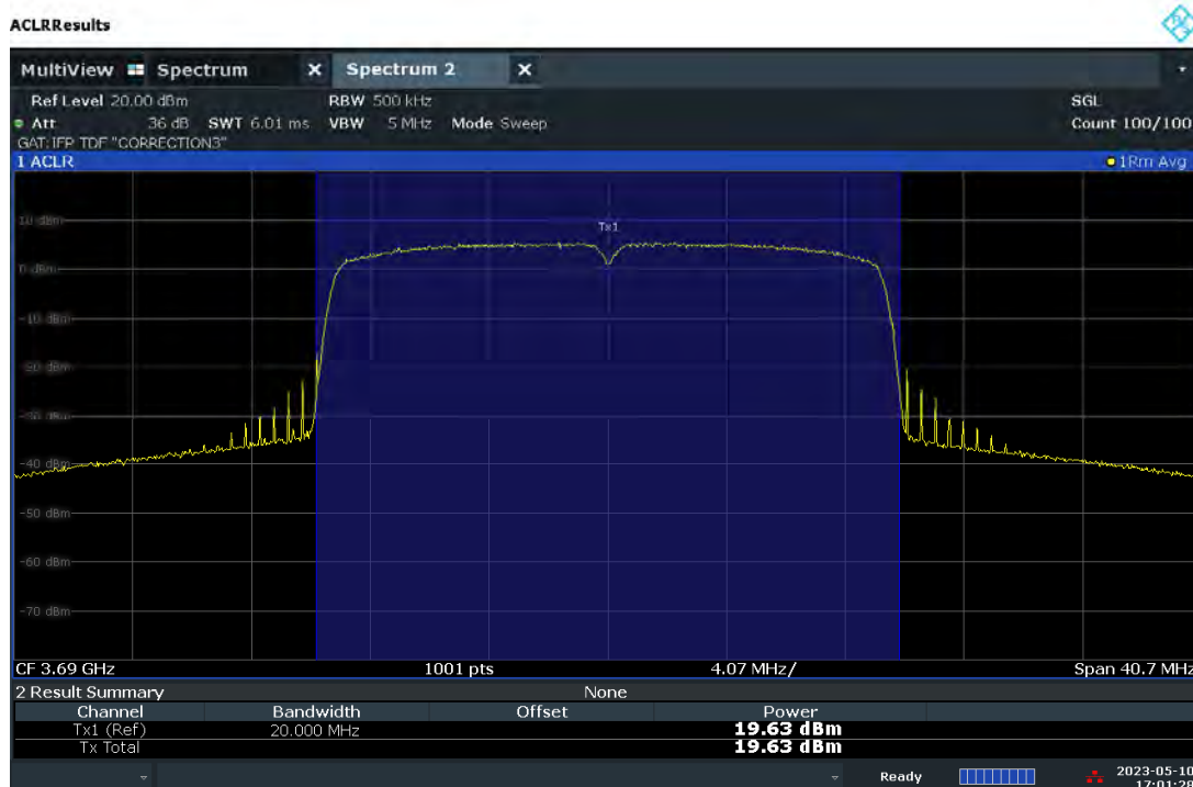
Plot 7.8 – Conducted Power Measurement – 20MHz BW, High Channel, 256QAM – Ch.A
