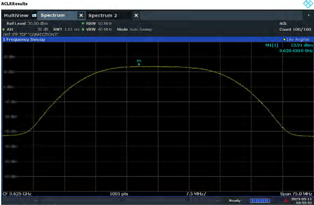
Plot 7.75. Conducted Power / 10MHz (30MHz 64QAM, Mid Channel – Ch.A)
