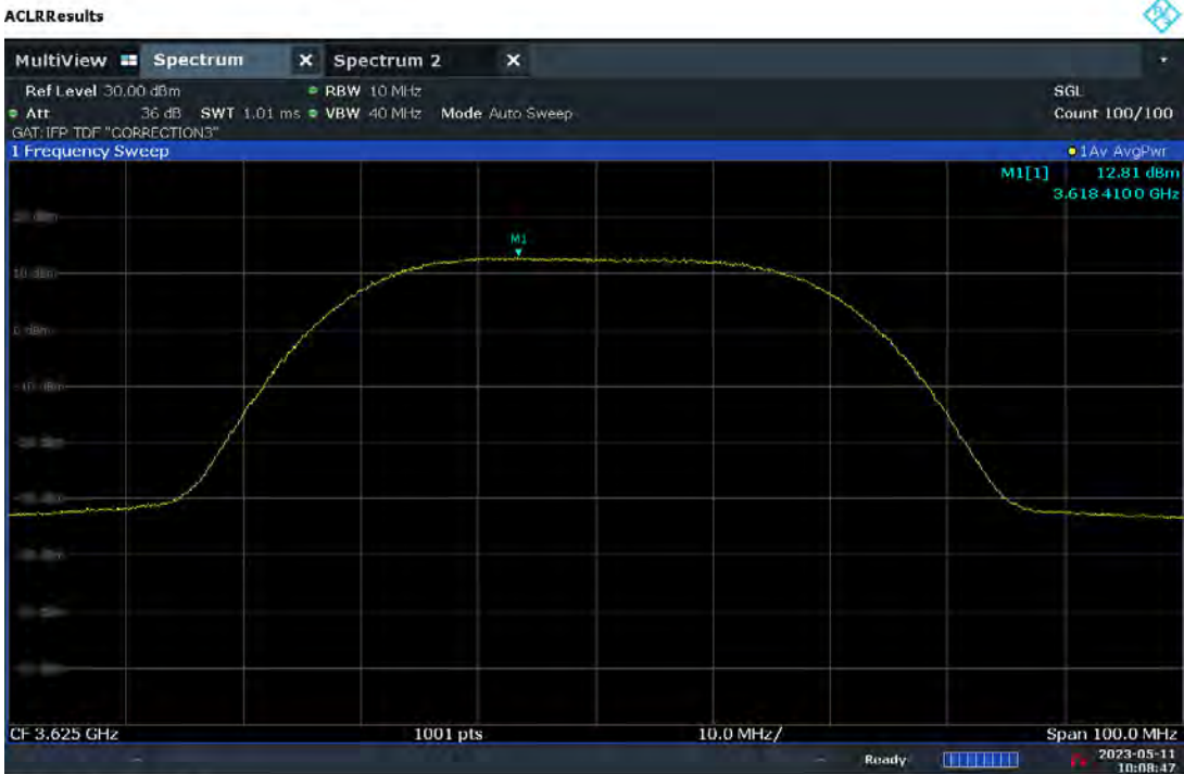
Plot 7.80. Conducted Power / 10MHz (40MHz 256QAM, Mid Channel – Ch.A)
