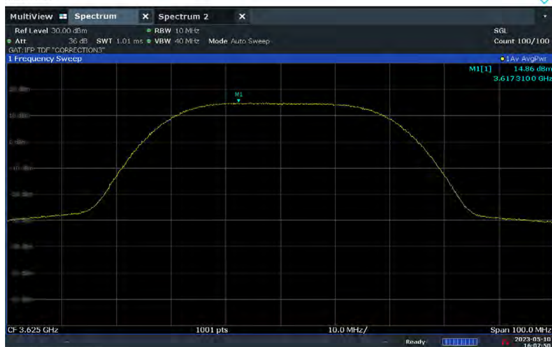
Plot 7.94. Conducted Power / 10MHz (40MHz 16QAM, Mid Channel – Ch.B)
