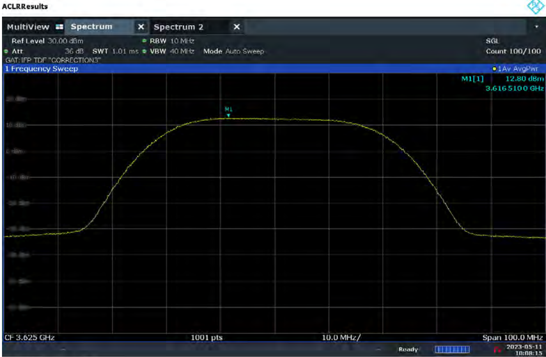
Plot 7.79. Conducted Power / 10MHz (40MHz 64QAM, Mid Channel – Ch.A)
