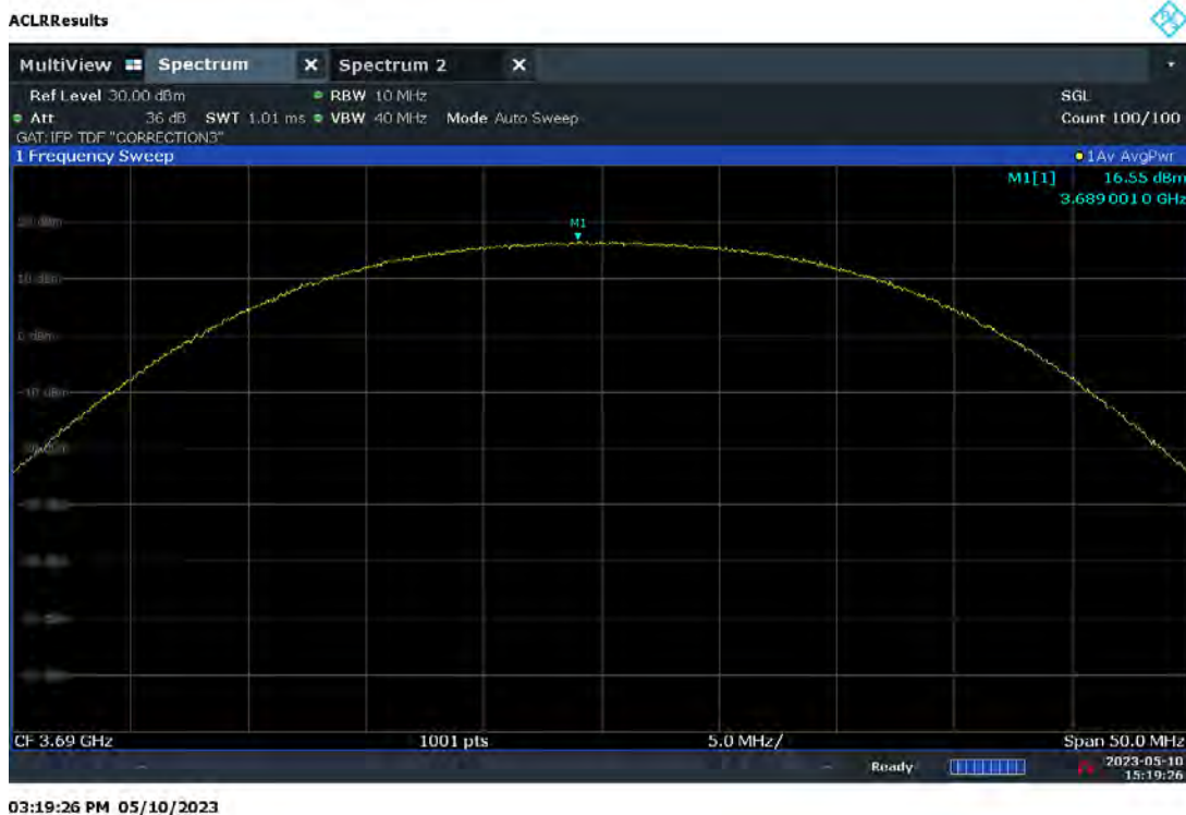
Plot 7.85. Conducted Power / 10MHz (20MHz QPSK, High Channel – Ch.B)
