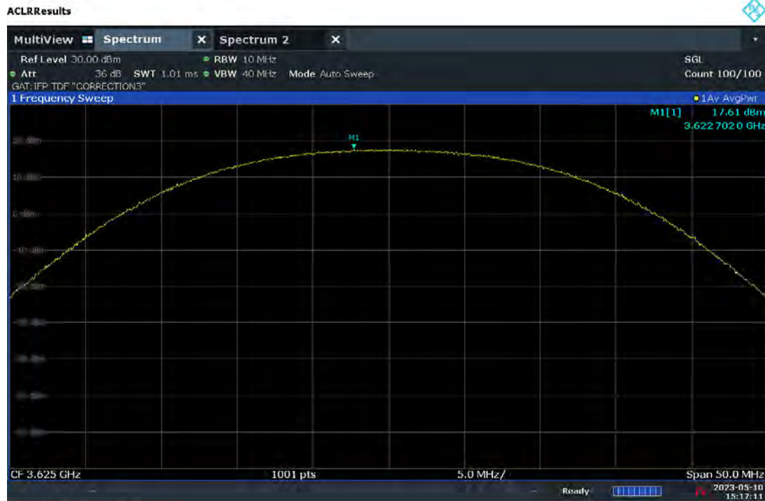
Plot 7.87. Conducted Power / 10MHz (20MHz 64QAM, Mid Channel – Ch.B)
