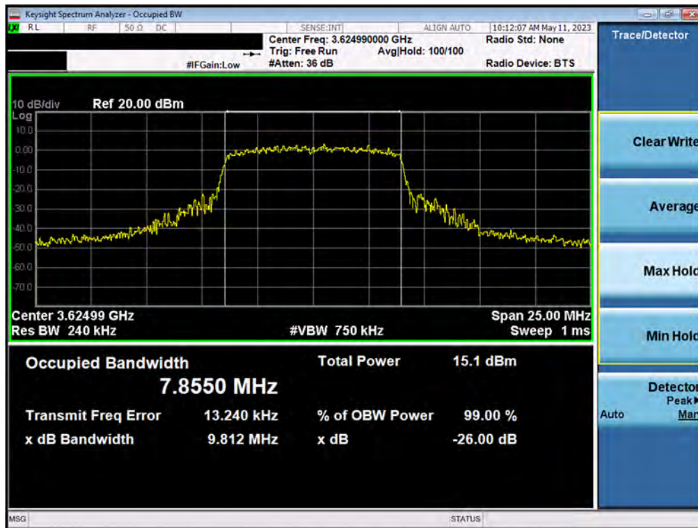
Plot 7.62. Occupied Bandwidth Plot (10MHz 16-QAM – Ch.B)
