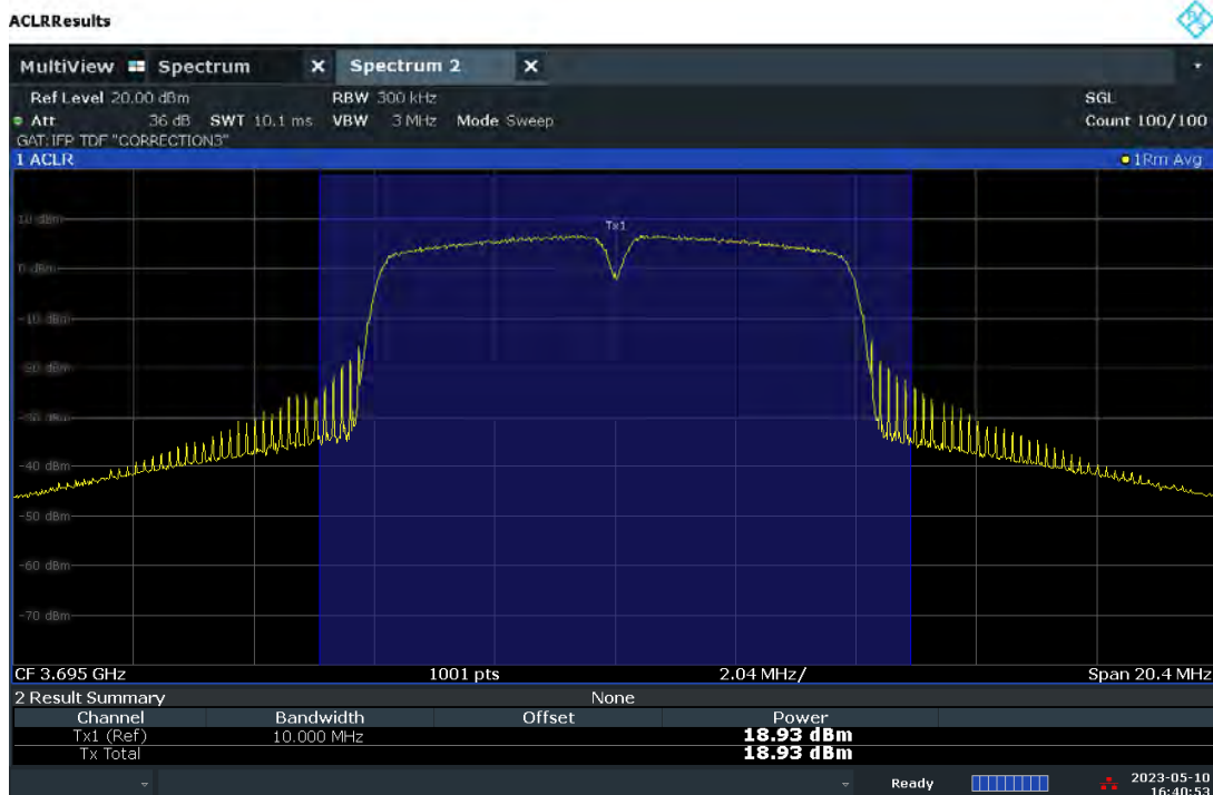
Plot 7.2 – Conducted Power Measurement – 10MHz BW, High Channel, 16QAM – Ch.A
