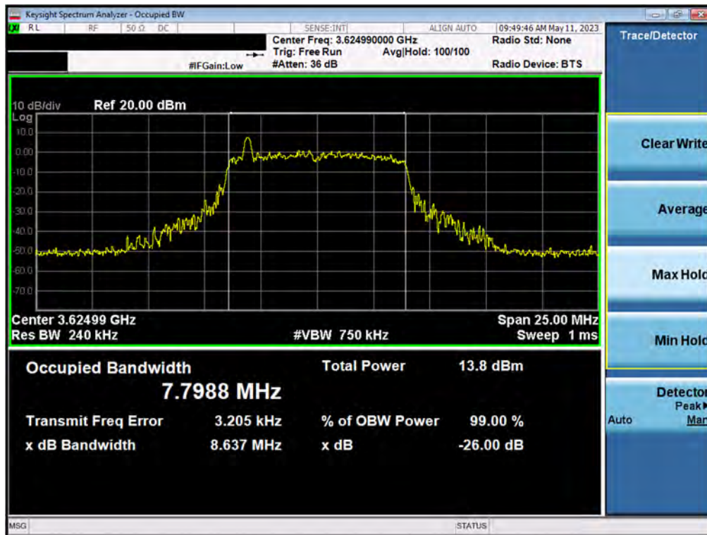
Plot 7.48. Occupied Bandwidth Plot (10MHz 256-QAM – Ch.A)
