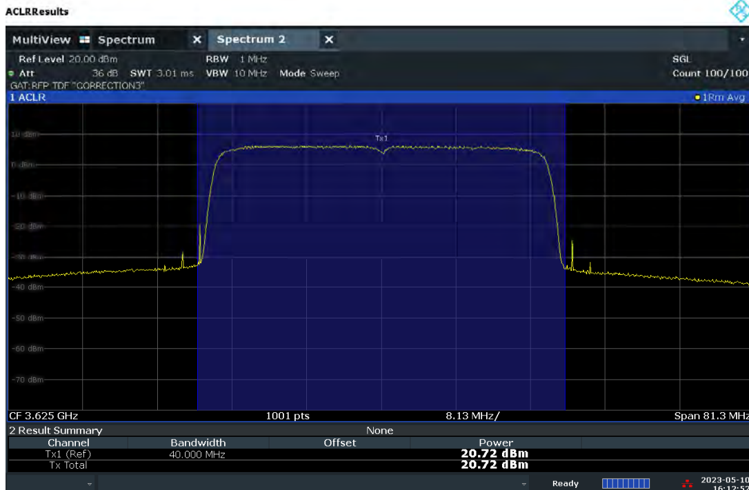
Plot 7.31 – Conducted Power Measurement – 40MHz BW, Mid Channel, 64QAM – Ch.B
