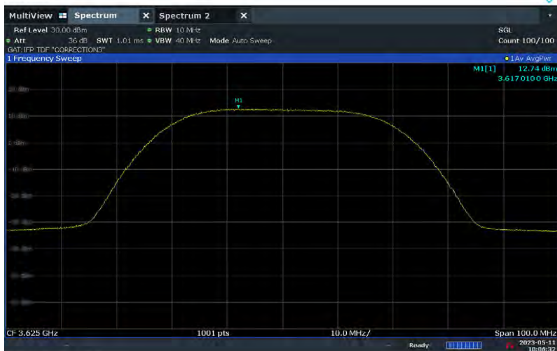
Plot 7.77. Conducted Power / 10MHz (40MHz QPSK, Mid Channel – Ch.A)
