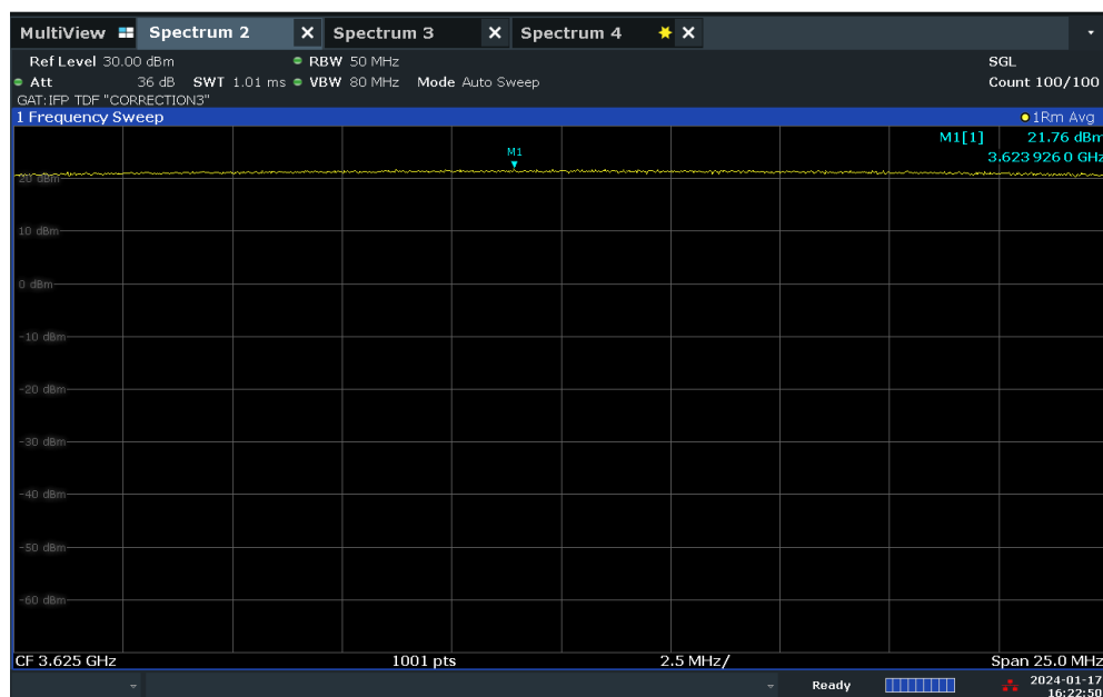
Plot 7.18 – Conducted Power Measurement – 10MHz BW, Mid Channel, 16QAM – ANT2
