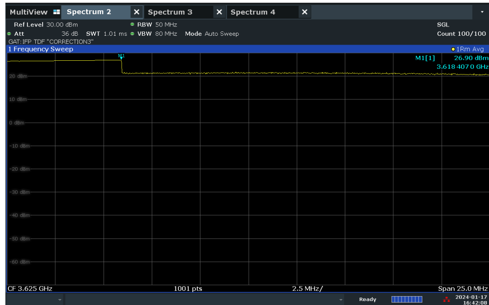
Plot 7.3 – Conducted Power Measurement – 10MHz BW, Mid Channel, 64QAM – ANT1
