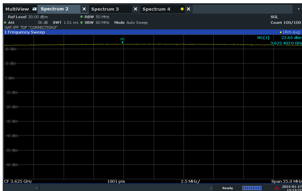
Plot 7.17 – Conducted Power Measurement – 10MHz BW, Mid Channel, QPSK – ANT2
