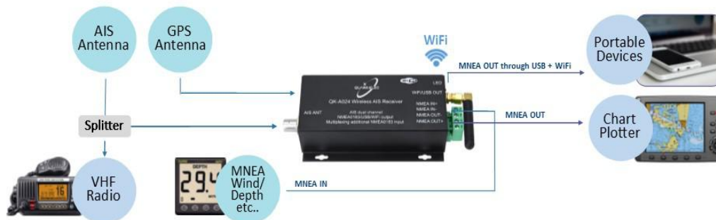
Figure 1 QK-A024/26 Connection Diagram
