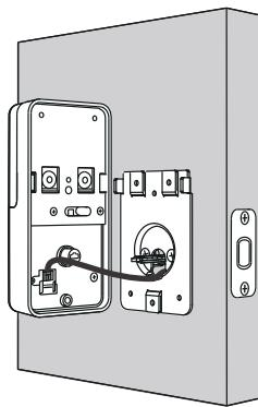
B. Align the interior panel with the cylinder for installation. After pressing the panel onto the door surface, manually turn the knob to ensure that the latch can extend and retract smoothly.
