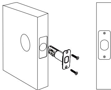
C. Install the strike plate on the door frame.
