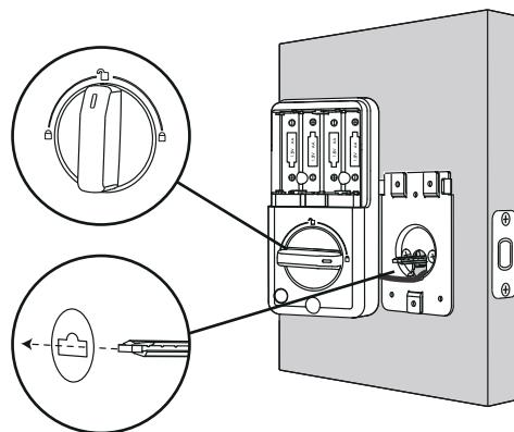
C. Secure the interior panel screws and install the battery.
