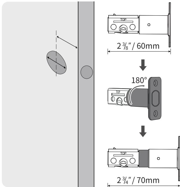
B. Insert and screw the deadbolt into the doorframe.
