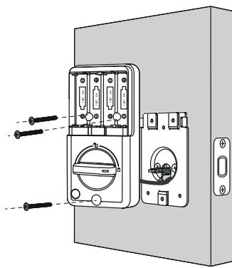
D. Install the 4 AA batteries provided with the correct polarity.
