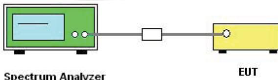
The EUT is coupled to the Spectrum Analyzer; the RF load attached to the EUT antenna terminal is 50Ohm; the path loss as the factor is calibrated to correct the reading. Make the measurement with the spectrum analyzer's resolution bandwidth(RBW) = 100 kHz. In order to make an accurate measurement, set the span greater than RBW.
