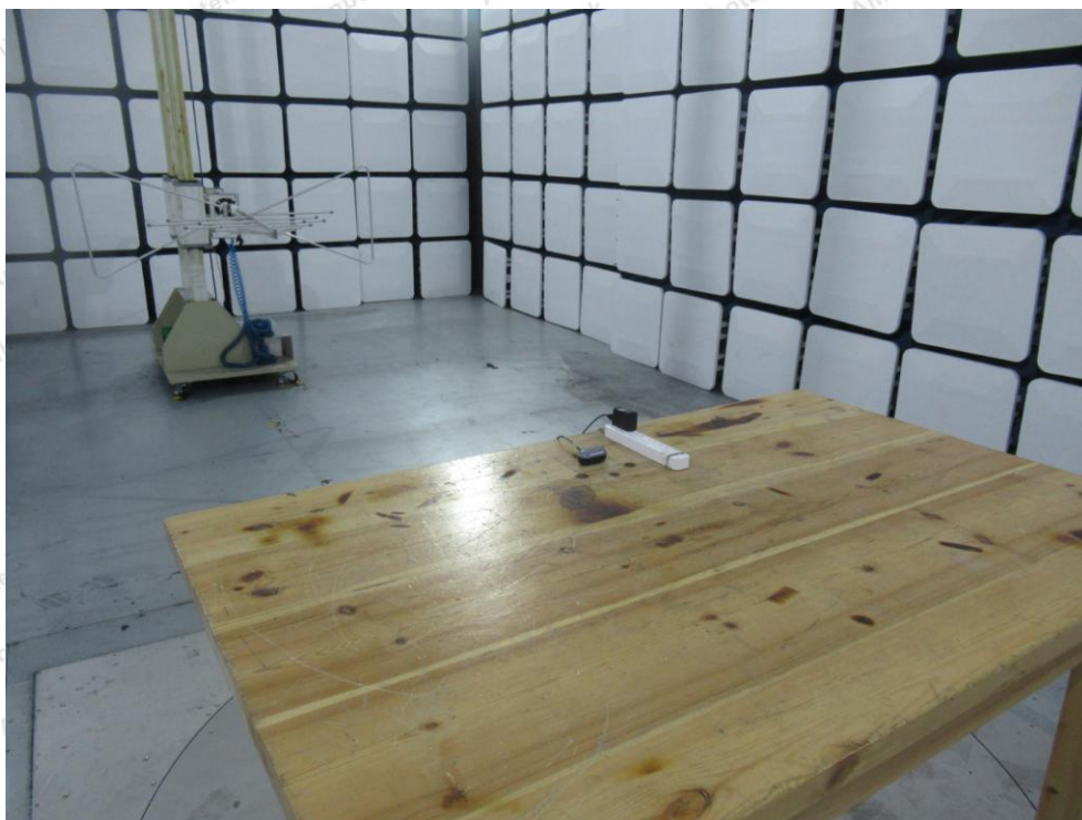
Photo of Radiation Emission Test
