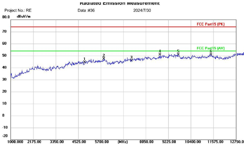
Site: Polarization: **Vertical** Temperature: (C)
