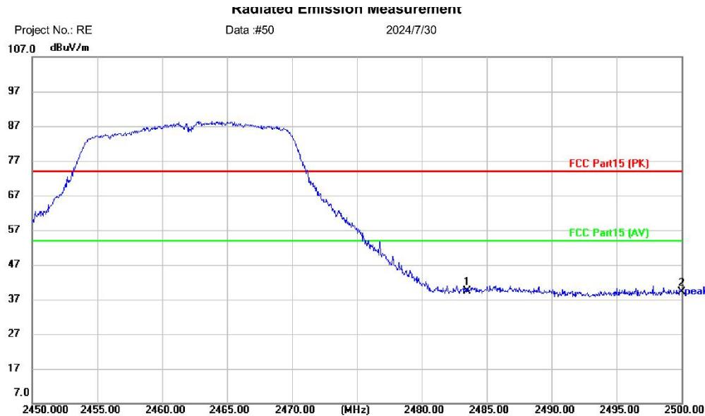
Site: Limit: FCC Part15 (PK) EUT: PanoX V3 M/N: PIP225 Mode: 2.4G G TX 2462 Note: Polarization: **Vertical** Power: Temperature: (C) Humidity: %RH
