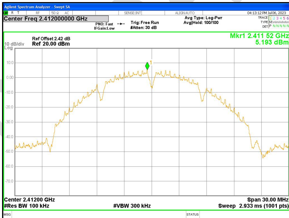
Band Edge NVNT b 2412MHz Ant2 Emission
