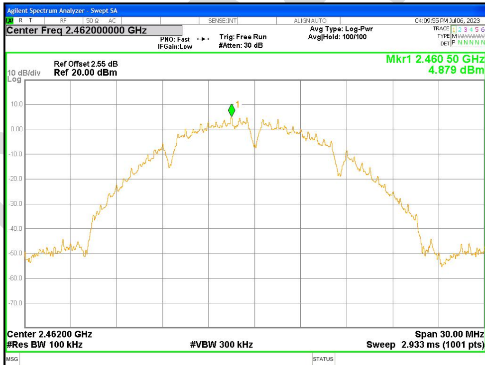
Band Edge NVNT b 2462MHz Ant1 Emission
