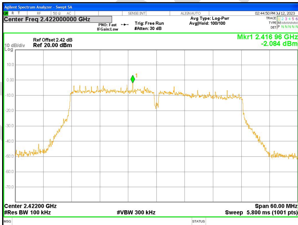
Band Edge NVNT n40 2422MHz Ant2 Emission
