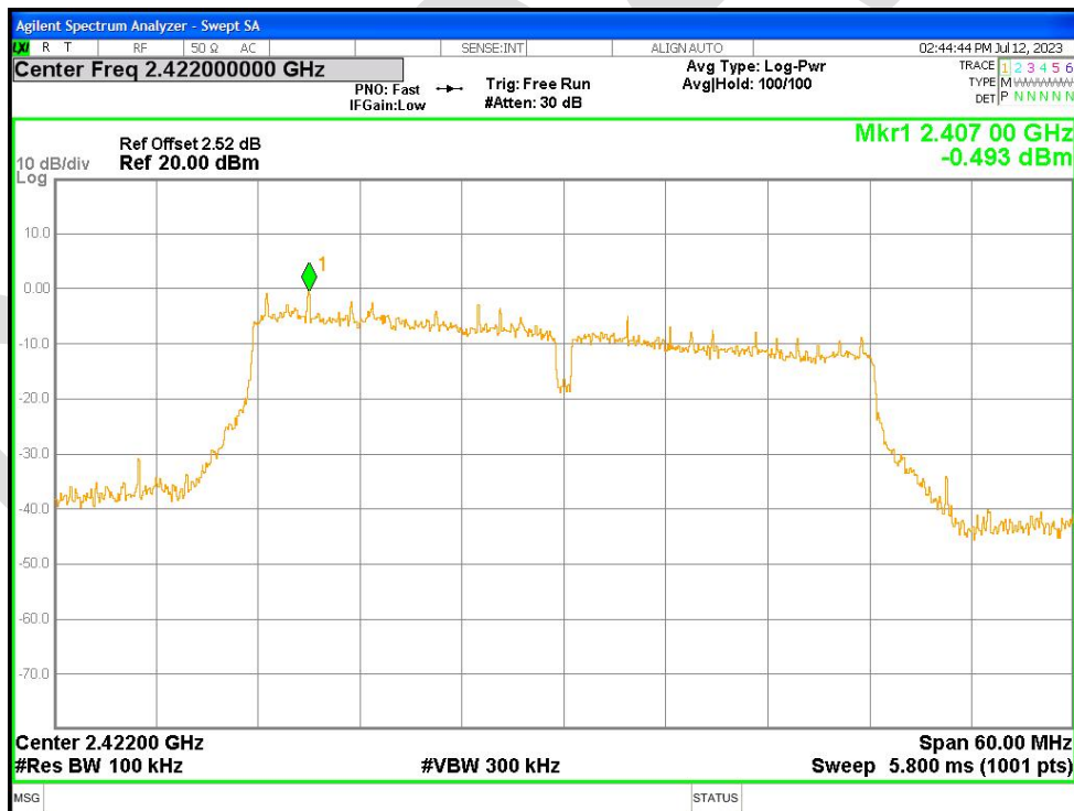
Band Edge NVNT n40 2422MHz Ant1 Emission
