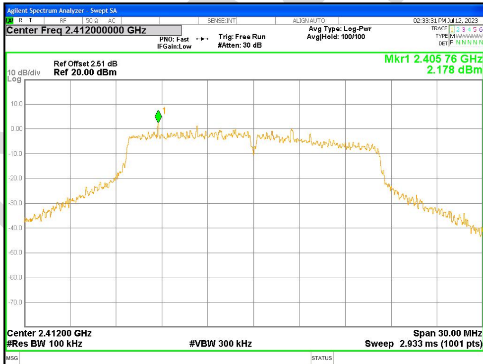
Band Edge NVNT g 2412MHz Ant1 Emission
