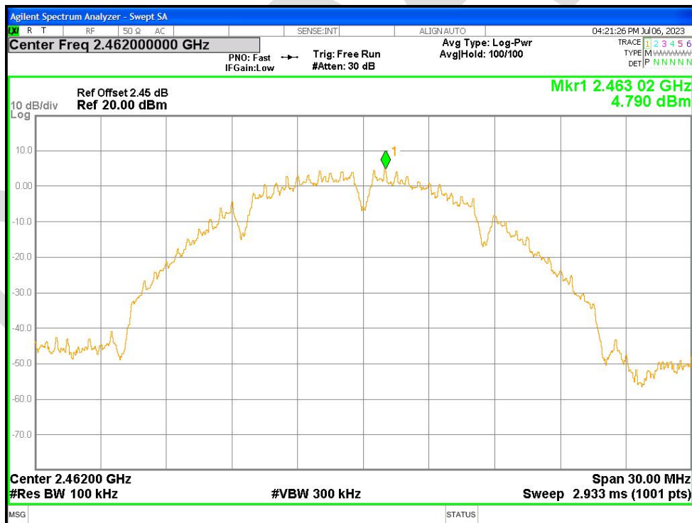
Band Edge NVNT b 2462MHz Ant2 Emission
