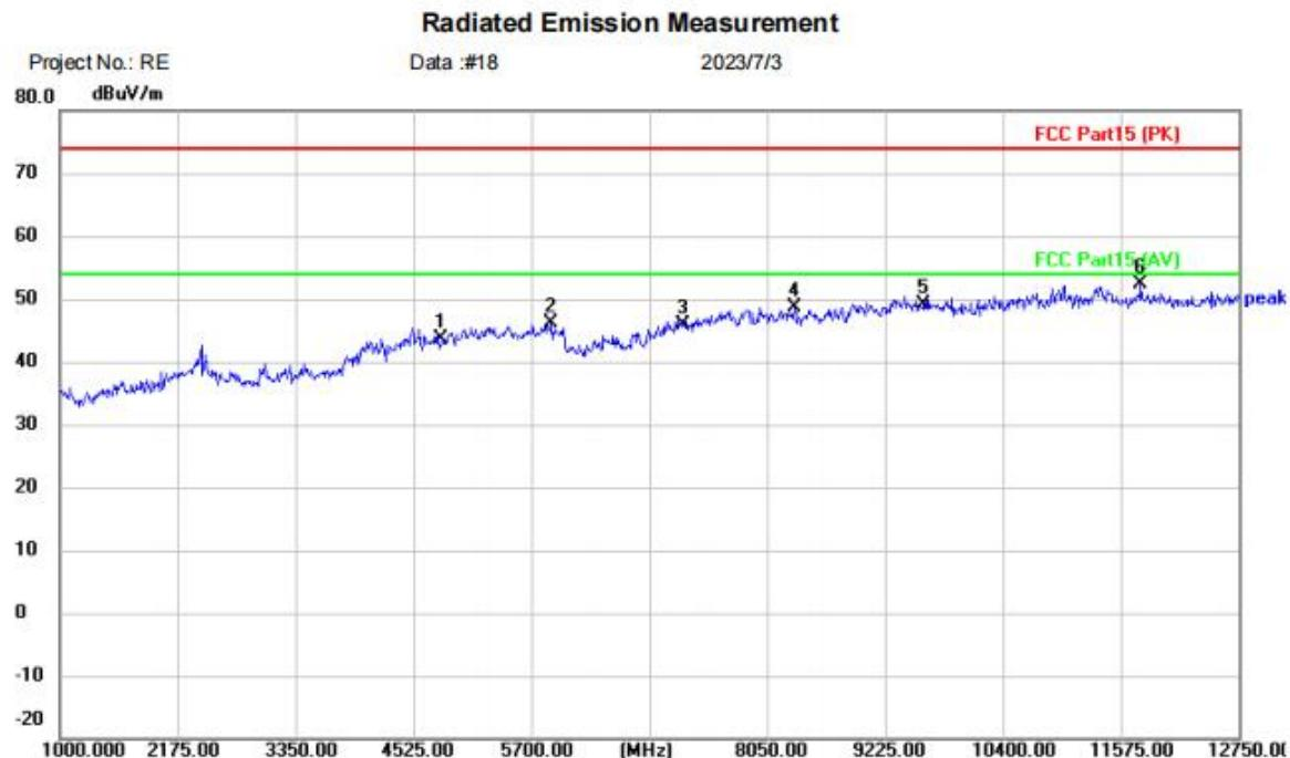
Site: Limit: FCC Part15 (PK) EUT: PANOX V2 M/N: PIP223 Mode: BLE 1 M TX-L Note: Polarization: **Vertical** Power: Temperature: (C) Humidity: %RH
