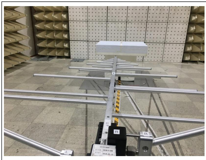
**- Photo of Radiated Spurious Emission Test (Above 1 GHz)**
