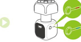
2 When charging the module, the LED beside the function button will be red. When charging is complete, the light will turn blue.
