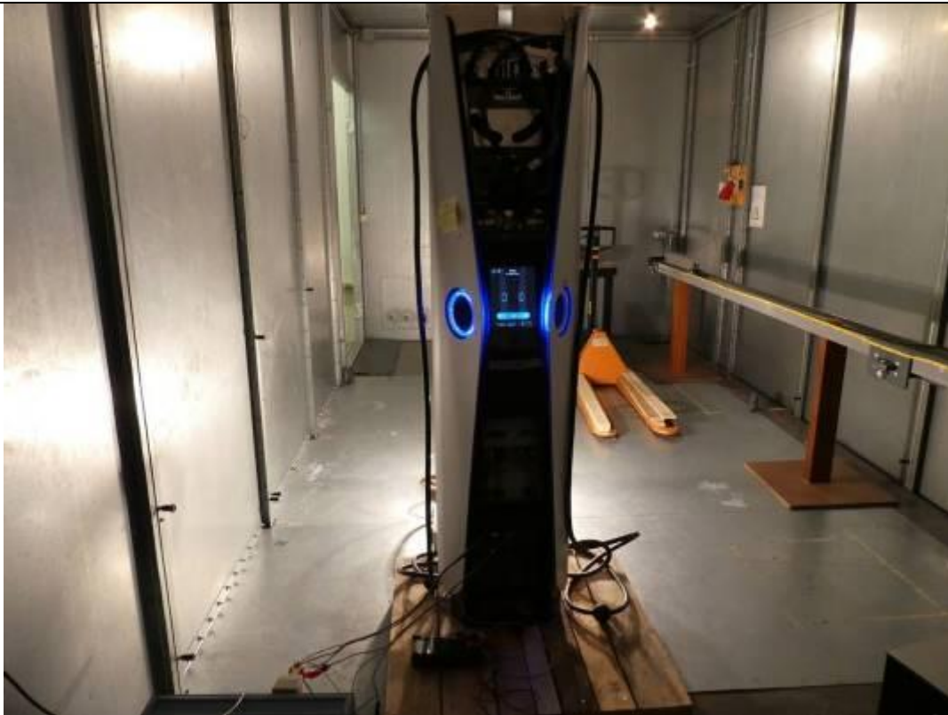
Figure B5: Conducted Emission Test setup Front
