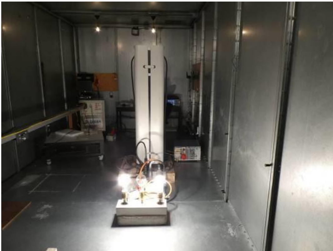
Figure B6: Conducted Emission Test Setup Rear
