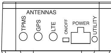
**NOTICE:** Ensure the cables are securely attached to the Gateway to avoid loosening due to vibration during vehicle operation.
