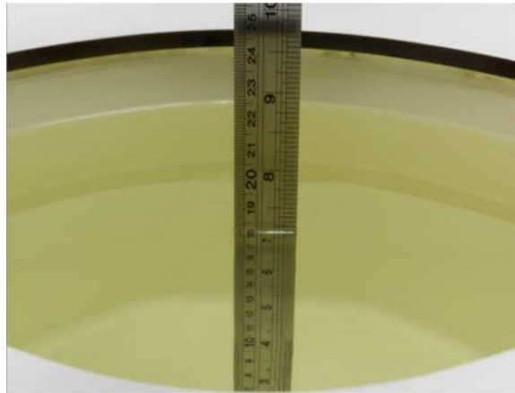
Fig 11.1 Photo of Liquid Height for Body SAR
