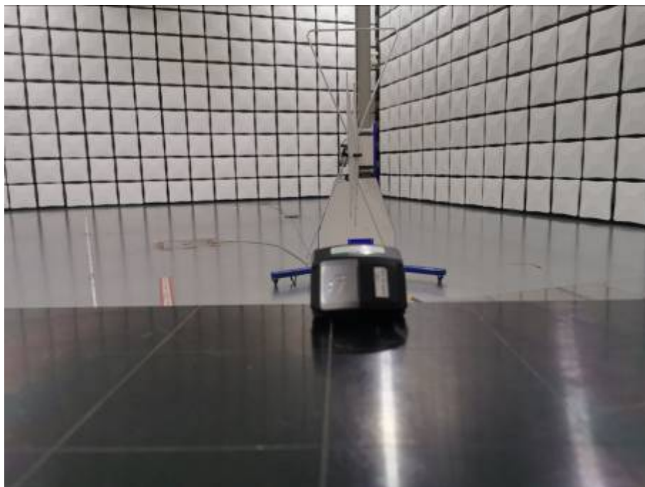
Radiated Emissions Test Setup (with charger) (30-1000MHz)
