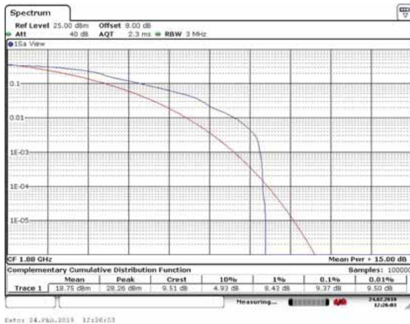
Peak-Average Ratio Plot(3MHz BW,16QAM,Band 2-mid Channel)
