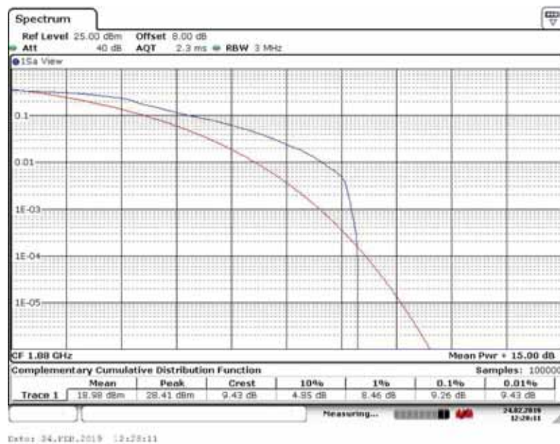
Peak-Average Ratio Plot(20MHz BW,16QAM,Band 2-mid Channel)
