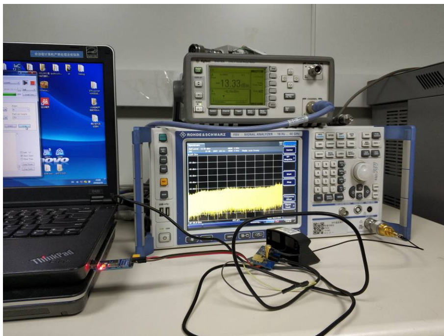
RF Conducted Test setup (BLE/WIFI)
