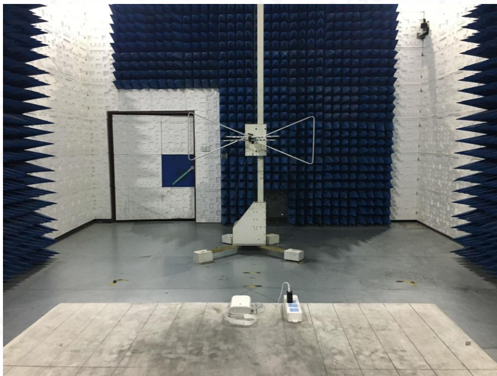
RADIATED EMISSION TEST SETUP ABOVE 1GHZ
