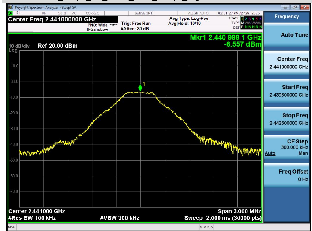
Test Graph BR ANT1 2441 1Mbps Reference Level
