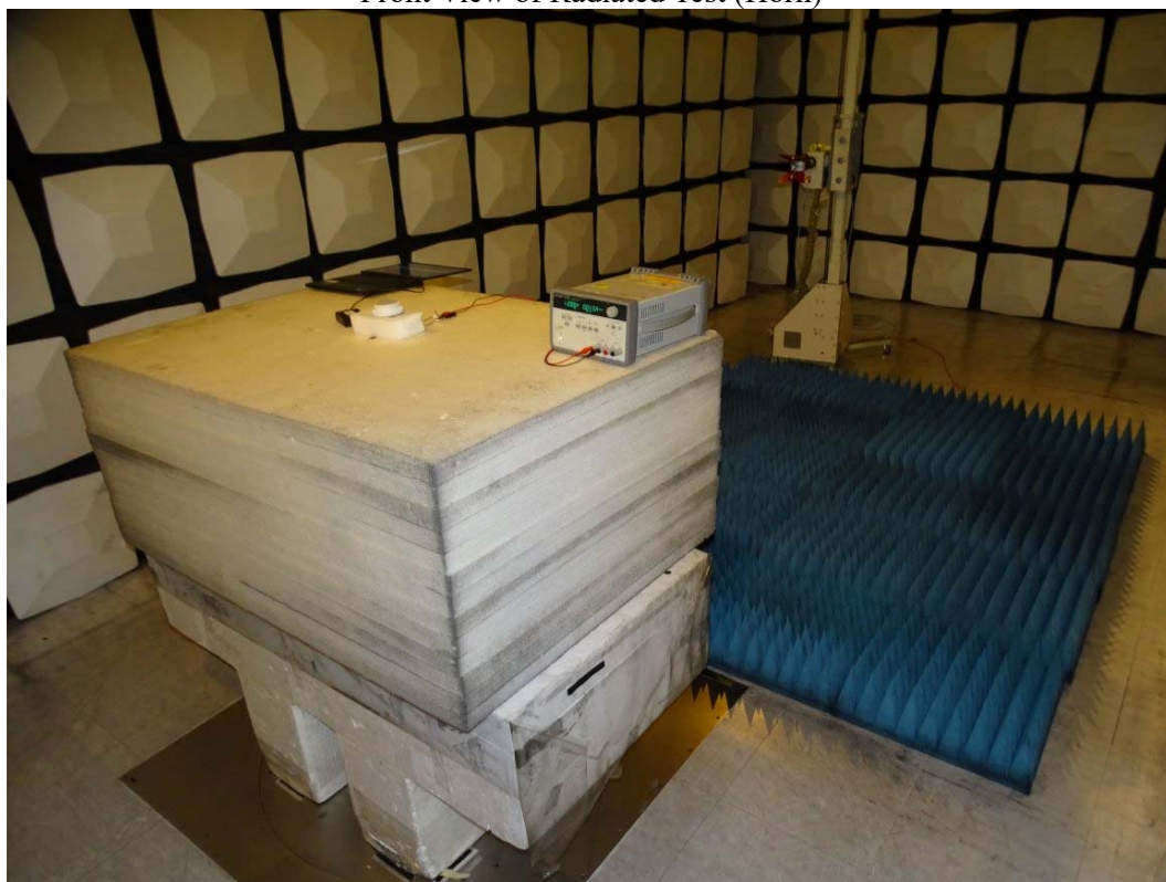
Front View of Radiated Test (Horn)
