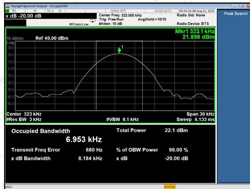
Note: The measured signal is Cw-like, adjusting the RBW per C63.10 would not be practical since measurement bandwidth will always follow the RBW. The RBW is set to 300 Hz to perform the occupied bandwidth test.
