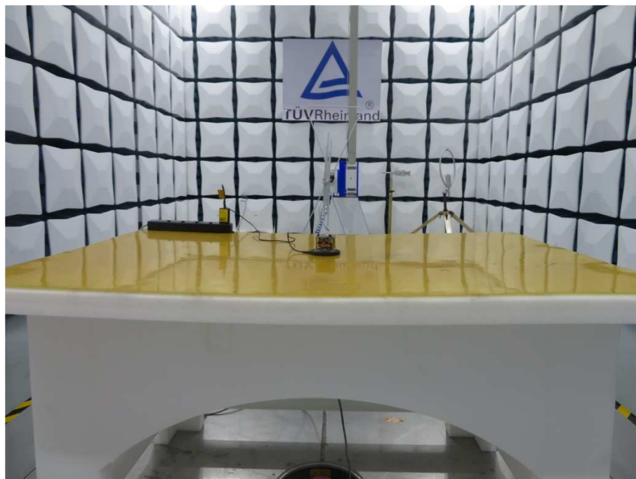
Photograph 2: Set-up for Radiated Spurious Emissions, above 30MHz
