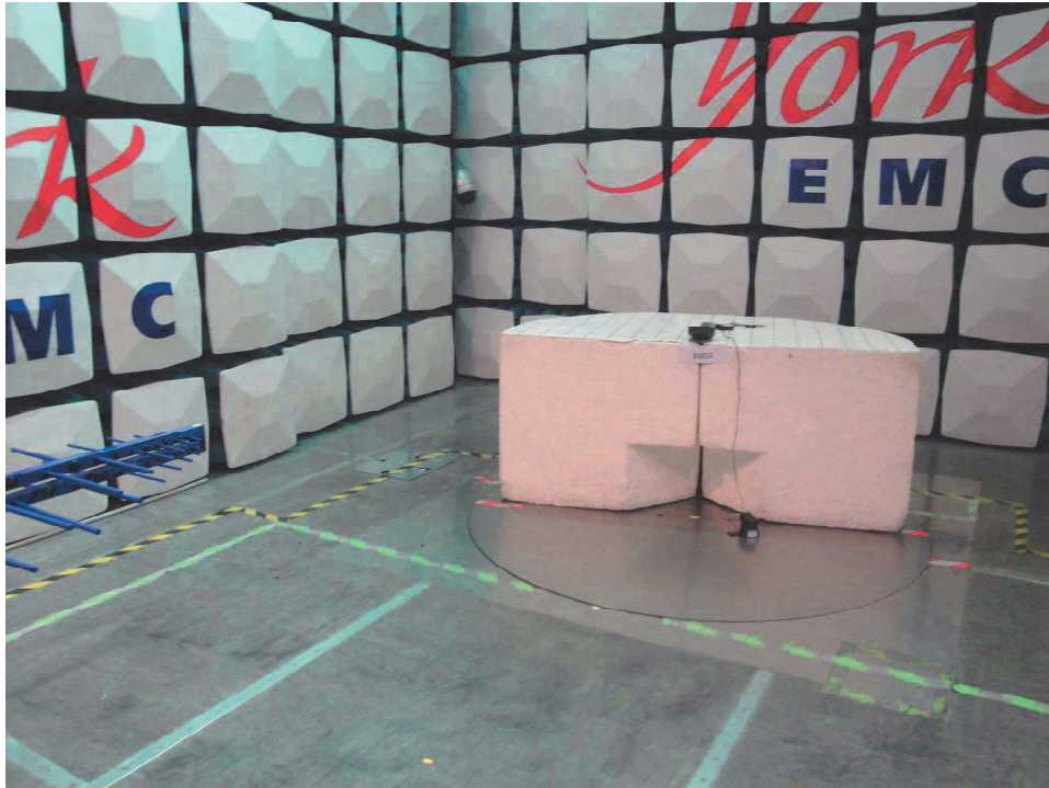
Photo 3: Radiated Emissions, 30MHz to 1GHz
