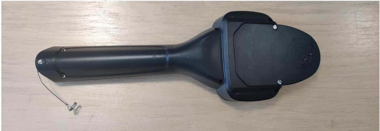
Battery cover: There is a single cover on the rear of the WAND Probe. This covers all internal components, including the battery
