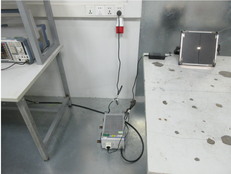
Photo of Power Line Conducted Emission Test
