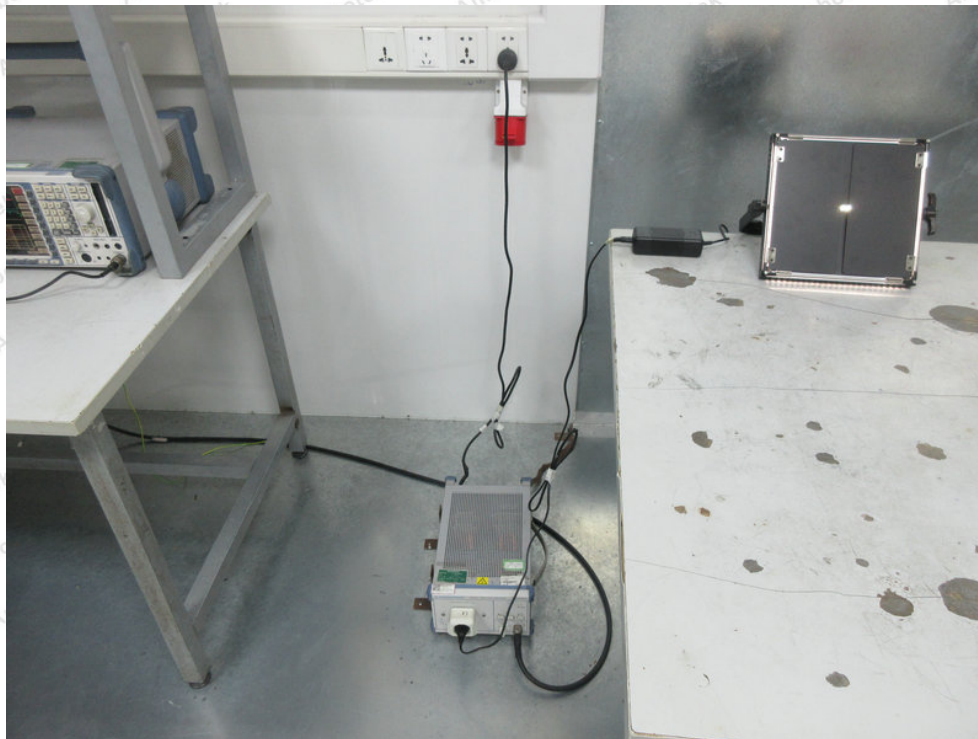
Photo of Power Line Conducted Emission Test
