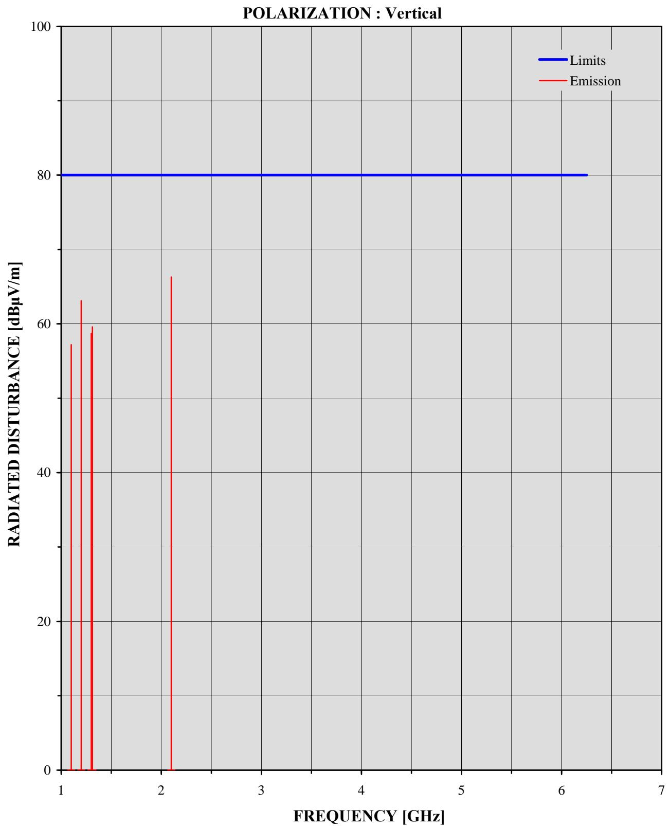
**Radiated Disturbance Measurements (1 GHz to 6.25 GHz)****Test Specification**
