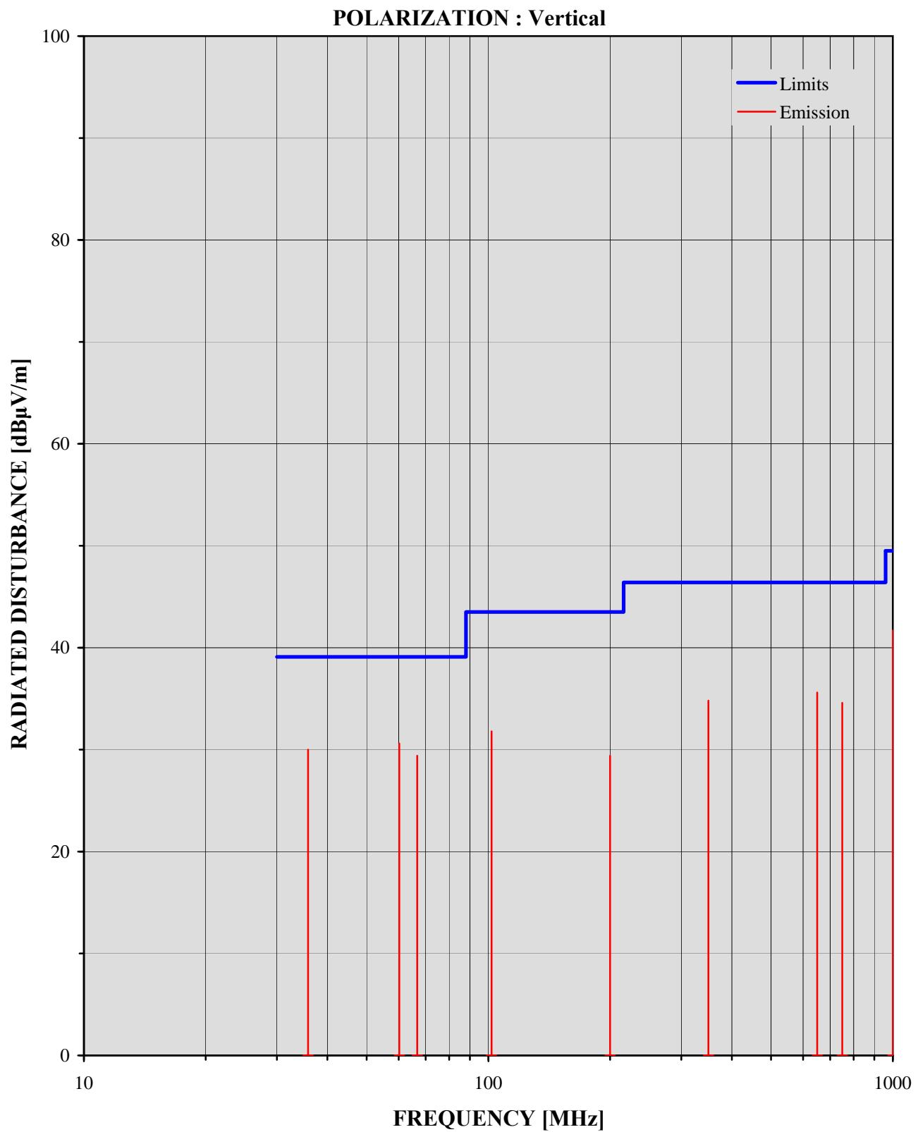
**Radiated Disturbance Measurements (30 MHz to 1000 MHz)****Test Specification**
