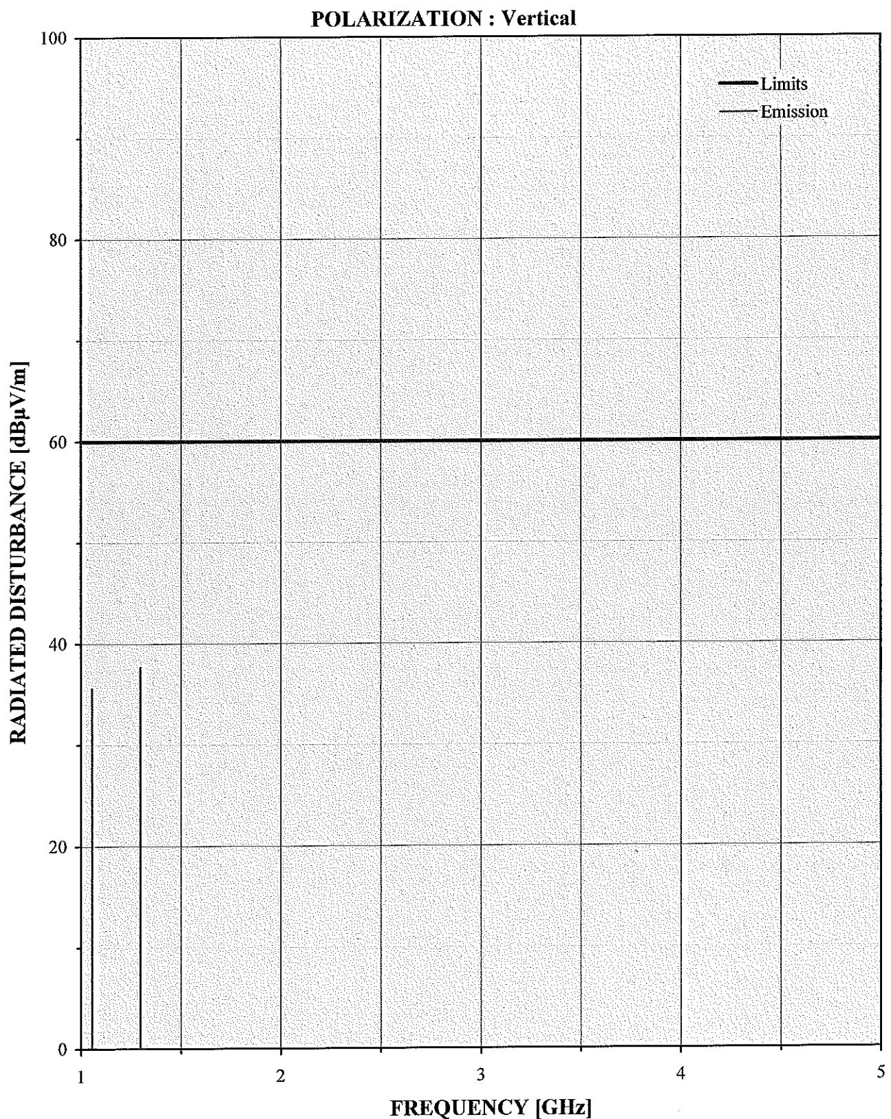
**Radiated Disturbance Measurements (1GHz to 5GHz)****Test Specification**
