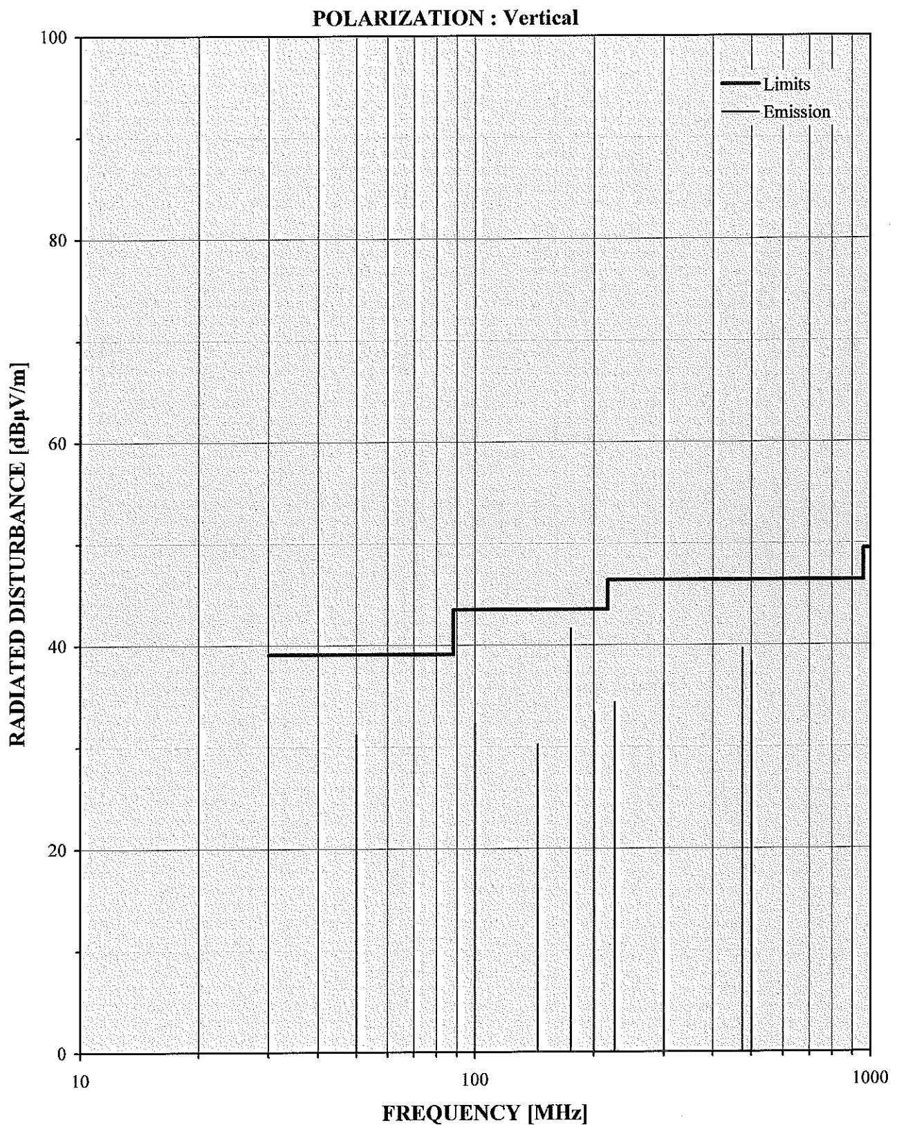
**Radiated Disturbance Measurements (30MHz to 1000MHz)****Test Specification**
