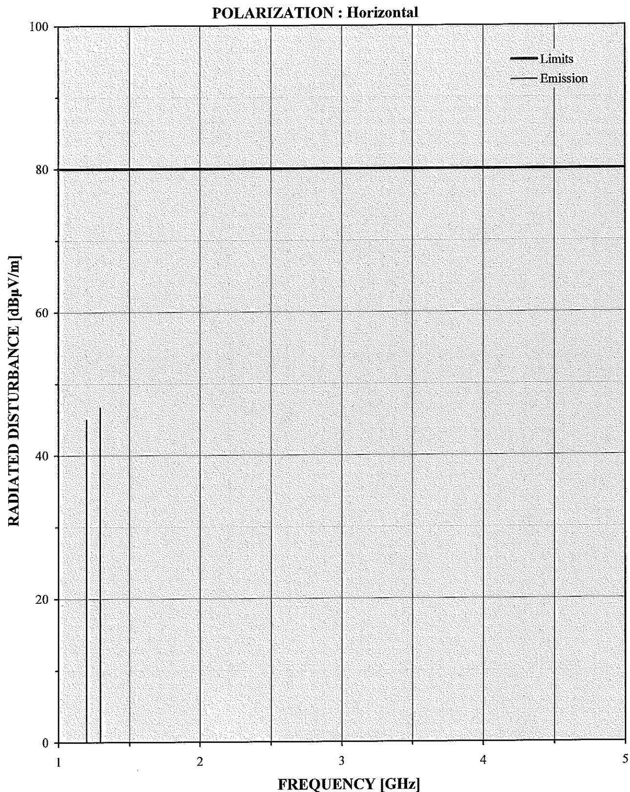
**Radiated Disturbance Measurements (1GHz to 5GHz)****Test Specification**
