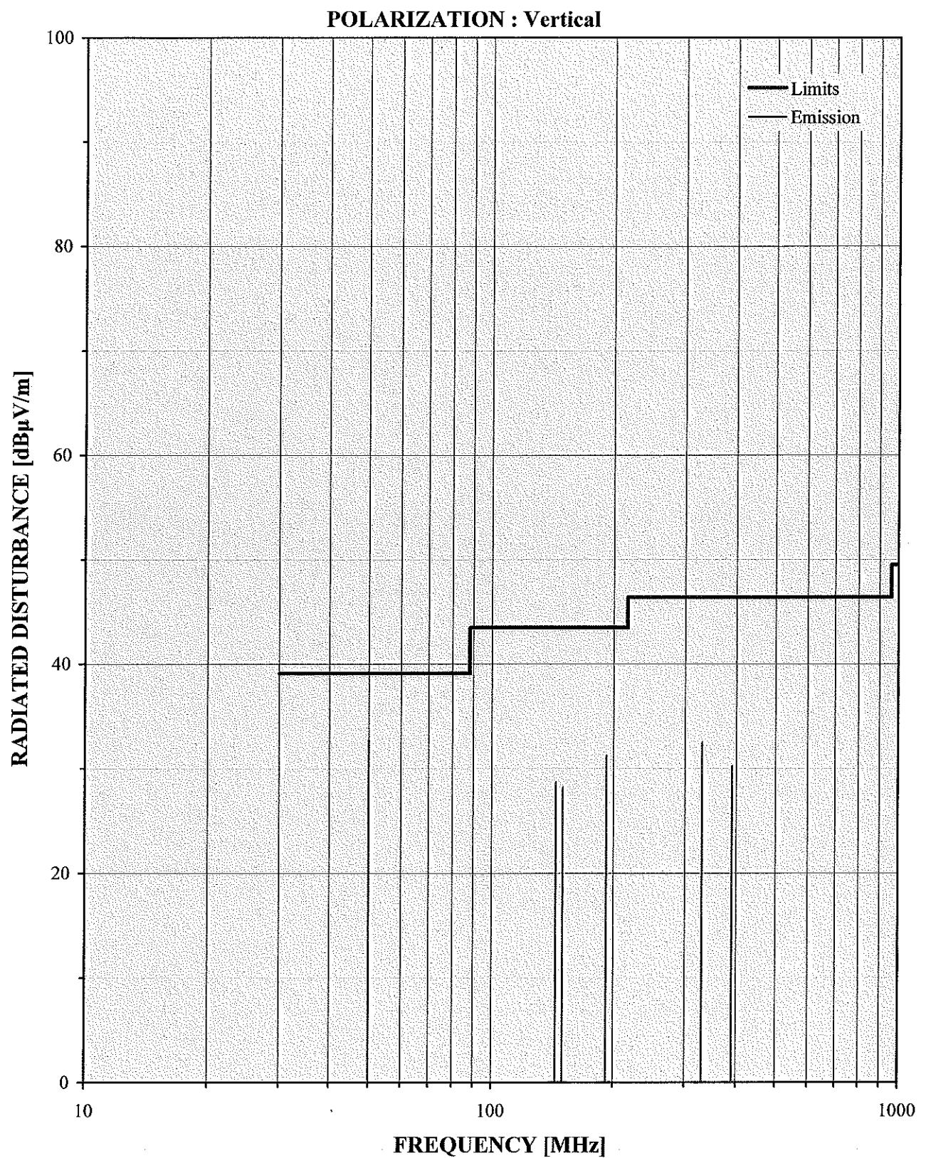
**Radiated Disturbance Measurements (30MHz to 1000MHz)****Test Specification**
