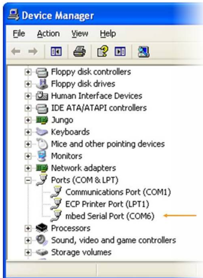
Figure 3. COM port associated with the PT7682W/PT7686W-SAOPTC0 HDK
