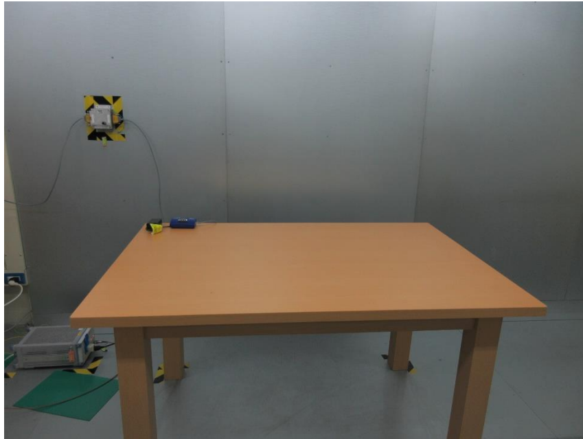
Photograph 1: Set-up for Conducted Emission (AC Mains)
